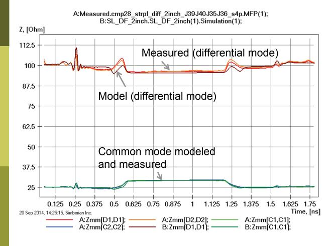
Model transitions have lower impedance due to no adjustments in trace width in polygonal section;
