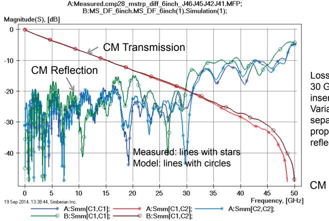
Loss of launch localization above 30 GHz explains additional insertion losses; Variation of trace width, separation and dielectric properties explains differences in reflection losses;
