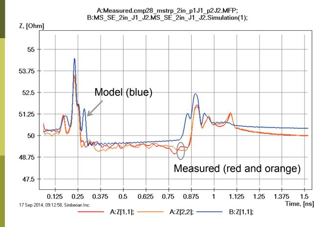
Variations of impedance along the traces visible here indicates that either trace width is varying or dielectric is inhomogeneous (or both); This is not accounted for in the model and explains differences in the reflection.
