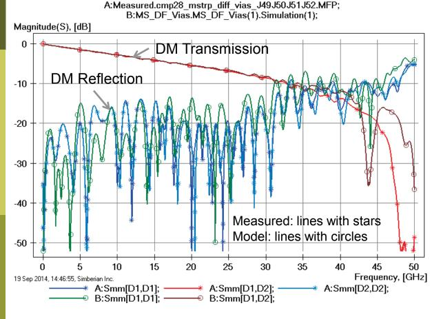
Loss of launch localization above 30 GHz explains additional insertion losses; Variation of trace width, separation and dielectric properties explains differences in reflection losses;
