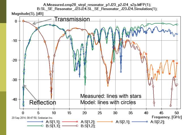
Loss of launch localization above 30 GHz explains additional insertion losses; Differences in back-drilling, variation of trace width and dielectric properties explains differences in reflection losses;
