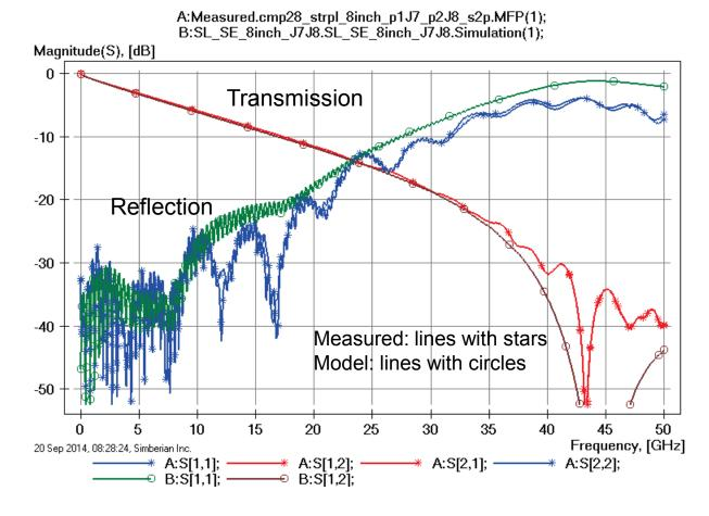
Loss of launch localization above 30 GHz explains additional insertion losses; Differences in back-drilling, variation of trace width and dielectric properties explains differences in reflection losses;
