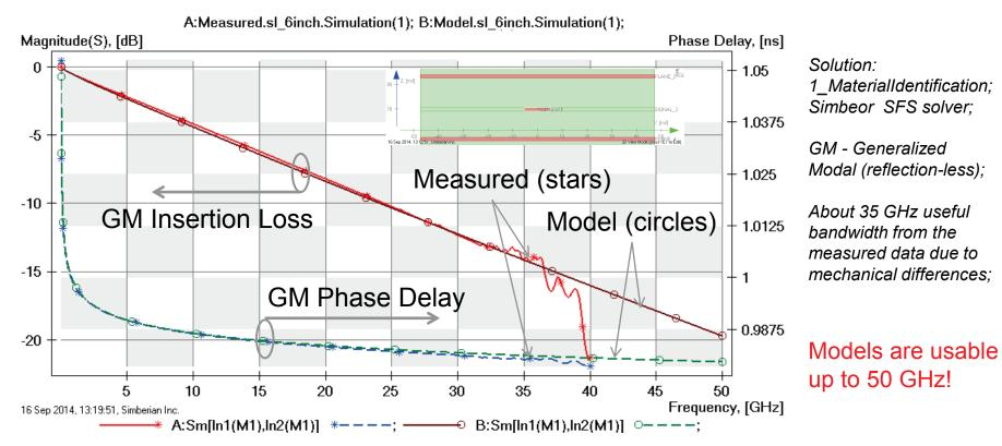
GMS parameters computed from S-parameters measured for 2 and 8 inch strip line segments (red and blue lines) and modeled for 6 inch strip line segment (brown and green lines): FR408HR model: Wideband Debye, Dk=3.815 (3.66), LT=0.0117 @ 1 GHz; Conductor roughness model: Modified Hammerstad, SR=0.4 um, RF=2;
