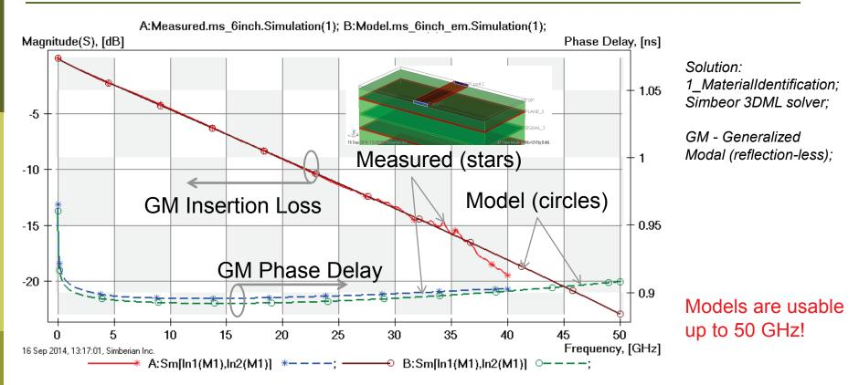
GMS parameters computed from S-parameters measured for 2 and 8 inch micro-strip line segments (red and blue lines) and modeled for 6 inch micro-strip line segment (brown and green lines): FR408HR model: Wideband Debye, Dk=3.815 (3.66), LT=0.0117 @ 1 GHz (same as for strip); Taiyo solder mask model: Wideband Debye, Dk=3.85 (3.9), LT=0.02 @ 1 GHz; Conductor roughness model: Modified Hammerstad, SR=0.4 um, RF=3.5;
