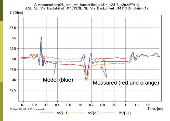
Variations of via back-drilling and trace geometry explains differences;
