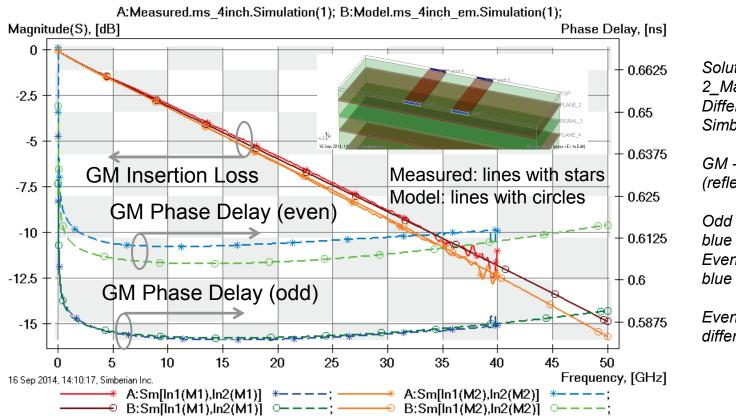
Solution: 2\_MaterialIdentification Differential; Simbeor 3DML solver;
