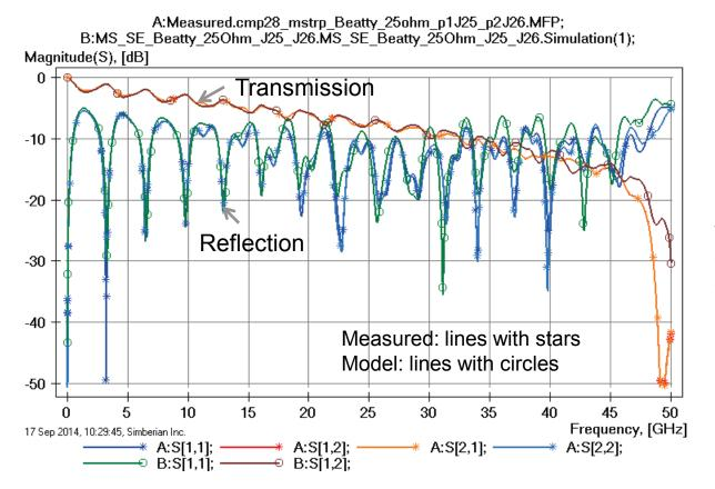
Loss of launch localization above 30 GHz explains additional insertion losses; Variation of trace width and dielectric properties explains differences in reflection losses;
