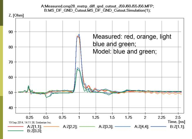
Model transitions have lower impedance due to no adjustments in trace width in the tapered polygonal section;
