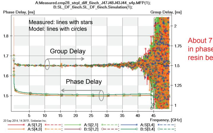
About 7 ps difference in phase delay due to resin between strips?
