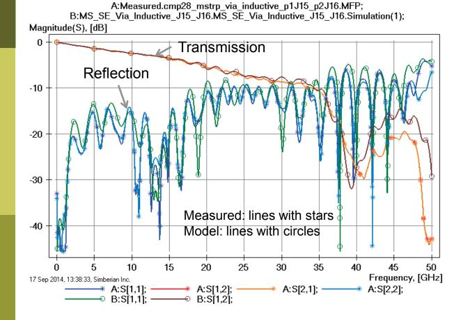
Loss of launch localization above 30 GHz explains additional insertion losses; Variation of trace width and dielectric properties explains differences in reflection losses;
