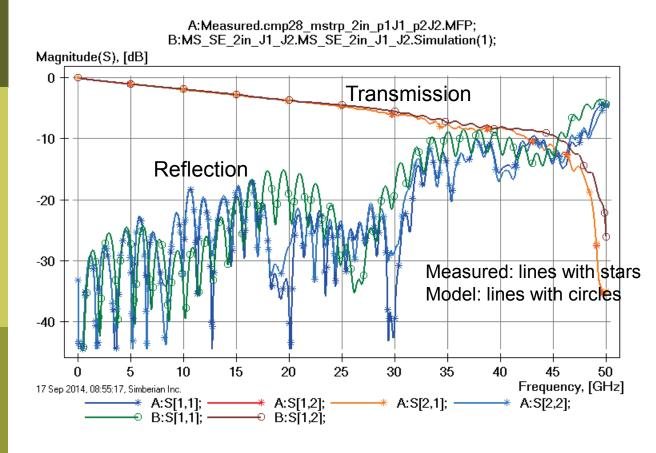
MS Launch looses the localization at about 30 GHz: Distance from signal via to stitching vias is about quarter of wavelength at 30 GHz – we cannot expect correlation above that frequency! Though, the impedance of the return path remains low due to plenty of stitching vias.
