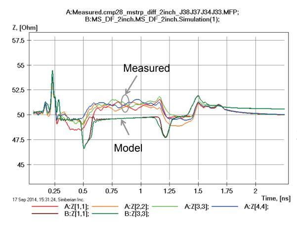
Model transitions have lower impedance due to no adjustments in trace width in the tapered polygonal section;
