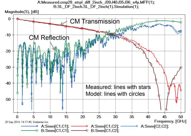
Loss of launch localization above 30 GHz explains additional insertion losses; Variations in back-drilling, trace width, separation and dielectric properties explains differences in reflection losses;
