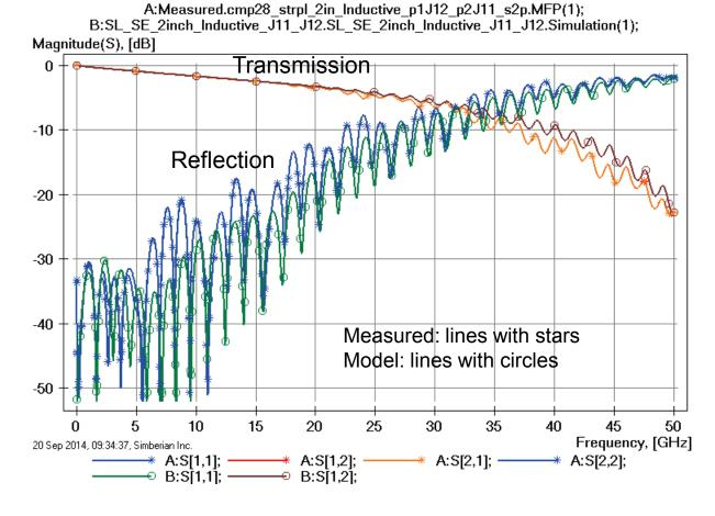
Variation of via geometry (back-drilling) explains differences both in insertion and reflection losses;
