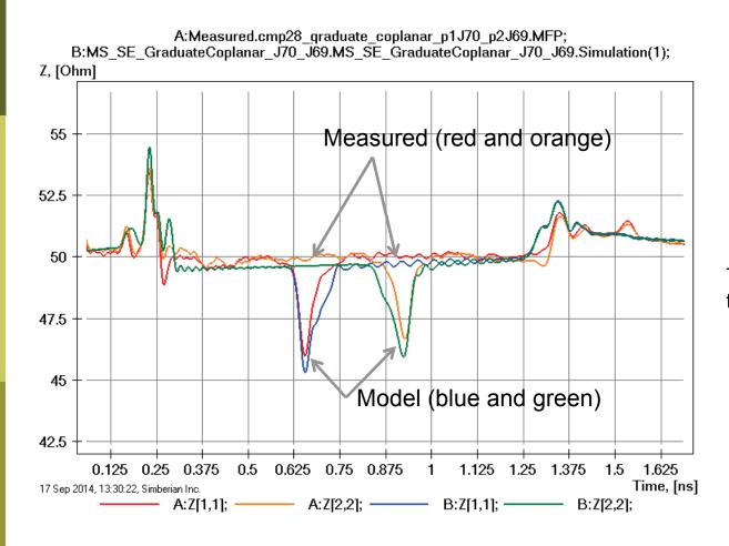
Trace width is not adjusted in the coplanar section;
