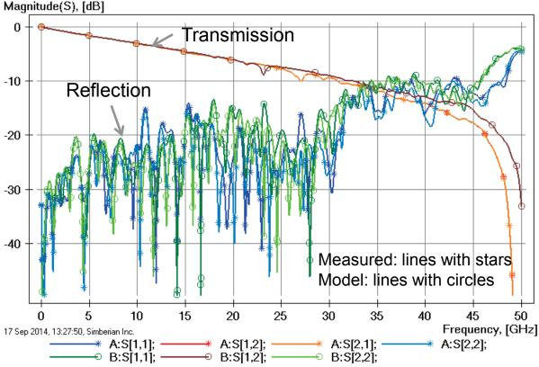
A:Measured.cmp28\_graduate\_coplanar\_p1J70\_p2J69.MFP; B:MS\_SE\_GraduateCoplanar\_J70\_J69.MS\_SE\_GraduateCoplanar\_J70\_J69.Simulation(1); Magnitude(S), [dB]
