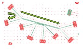
Loss of launch localization above 30 GHz explains additional insertion losses; Variation of trace width, separation and dielectric properties explains differences in reflection losses;
