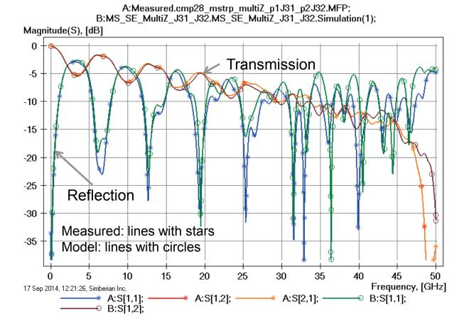
Variation of trace width and dielectric properties explains differences in reflection losses;
