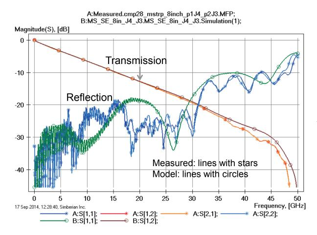
Loss of launch localization above 30 GHz explains additional insertion losses; Variation of trace width and dielectric properties explains differences in reflection losses;
