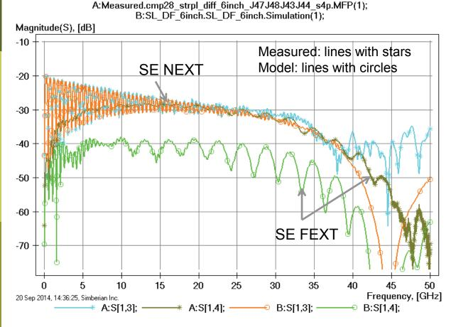
Difference in FEXT indicates inhomogeneity of dielectric (resin between strips);
