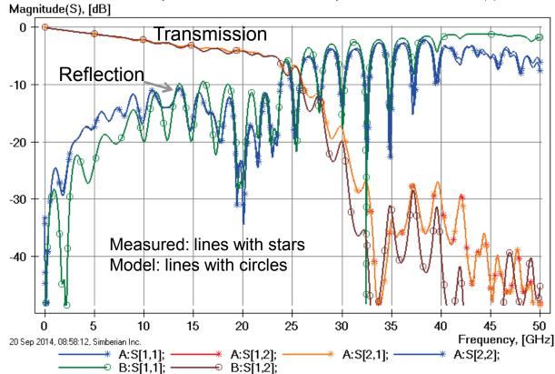
A:Measured.cmp28\_strpl\_via\_capacitive\_p1J18\_p2J17\_s2p.MFP(1); B:SL\_SE\_Via\_Capacitive\_J18J17.SL\_SE\_Via\_Capacitive\_J18J17.Simulation(1); |agnitude(S), [dB]
