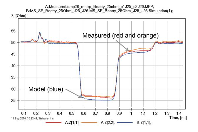
Impedance of the wider section is off (no adjustments);
