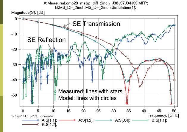
Difference in strip width and separation explains difference in transmission resonance; Variation of trace width and dielectric properties explains differences in reflection losses;
