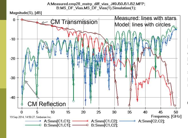
Loss of common mode localization above 15-20 GHz explains additional insertion losses;
