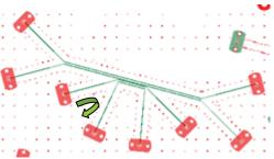
Model transitions have lower impedance due to no adjustments in trace width in polygonal section;
