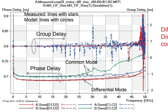
Differential mode is OK; Discrepancies in common above 20 GHz;
