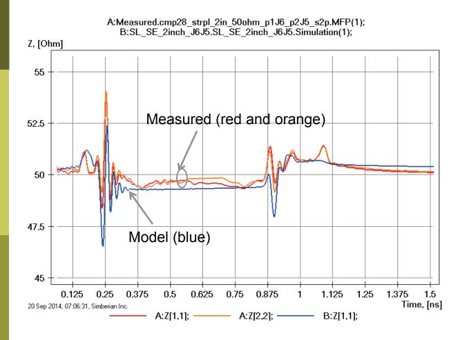
Variations of impedance along the traces visible here indicates that either trace width is varying or dielectric is inhomogeneous (or both); This is not accounted for in the model and explains differences in the reflection.
