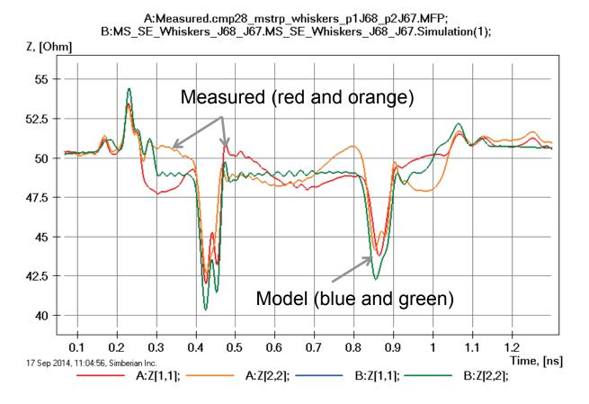
TRACES ON THE BOARD ARE NOT UNIFORM – it explains the differences above 20-25 GHz
