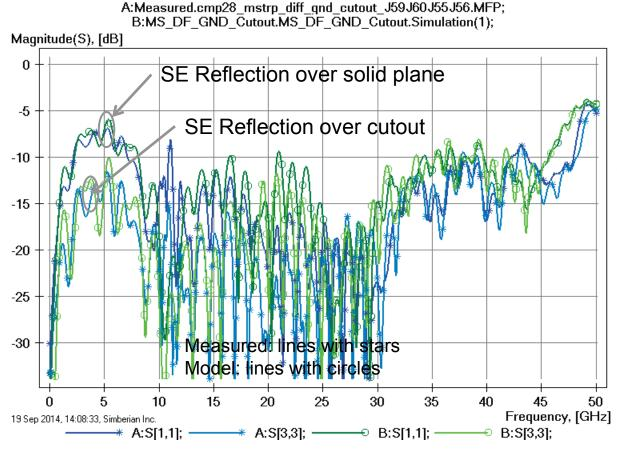
Difference in strip width, separation and dielectric properties explains difference in reflection;
