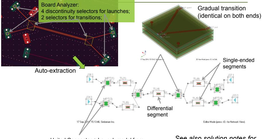
United Connector + Launch model from PCB/MS\_ConnectorAndLaunch
