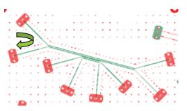
Model transitions have lower impedance due to no adjustments in trace width in polygonal section;
