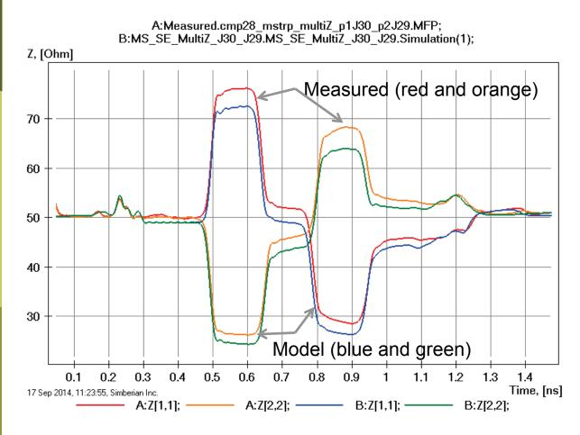
About 10% difference in wider lines; About 5% in narrow lines; No width adjustments in wider and narrower strips;
