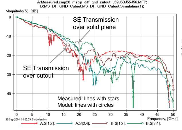
Difference in strip width and separation explains difference in transmission;
