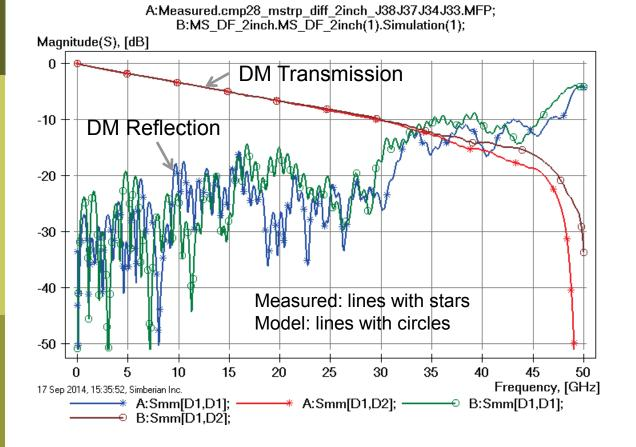
Loss of launch localization above 30 GHz explains additional insertion losses; Variation of trace width, separation and dielectric properties explains differences in reflection losses;
