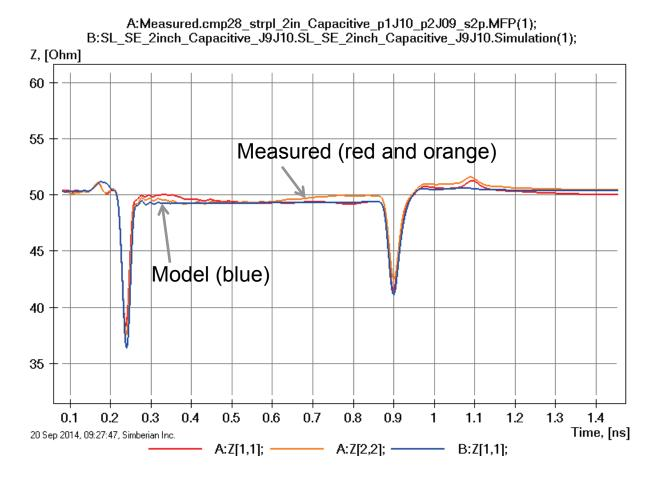
Variations of via back-drilling and trace geometry explains differences;
