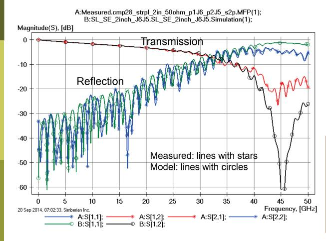
MS Launch looses the localization at about 30 GHz: Distance from signal via to stitching vias is about quarter of wavelength at 30 GHz – we cannot expect correlation above that frequency! Though, the impedance of the return path remains low due to plenty of stitching vias.
