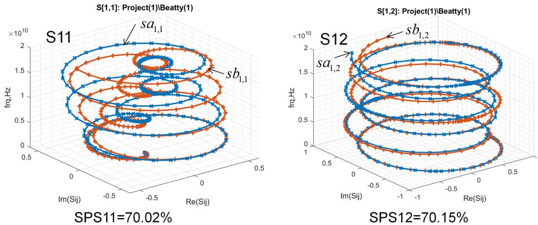
The plots do not have intersections as the polar plots and no jumps of angles as on Bode plots. The visual comparison is still difficult, but we can apply an image recognition technique to measure the similarity of the data sets. In particular, Modified Hausdorff Distance (MHD) can be used to measure the distance between the two data sets (S-parameters of 2 Beatty resonators in this case):
