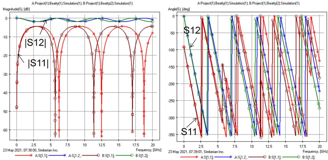
We can observe some shift of resonances in two structures, but it is difficult to make any conclusion on the angles – they are close at lower frequencies, but then deviate from each other. The jumps can be un-wrapped, but it is not always straightforward for measured data.
