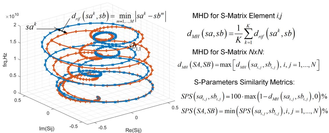
S-parameters similarity (SPS) measure with span from 0 (no similarity) to 100% (identical structures) can be introduced with the MHD computed for each element of matrix and for the whole matrix as shown on the picture above. **Very easy and straightforward – it is just a few lines of code in Matlab as shown in [4].**
