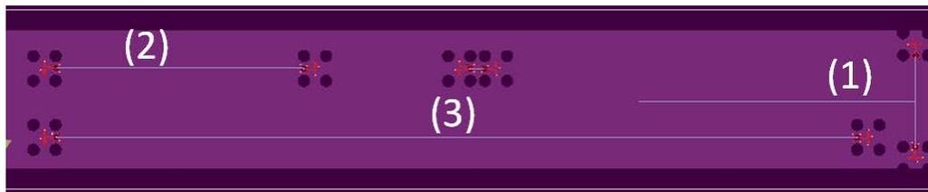
*Fig. 5.1. Example of test fixtures for Gamma-T process: T-resonator (1) and two transmission line segments (2) and (3).*
