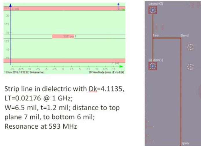
*Fig. 6.1. The original geometry of T-resonator.*
