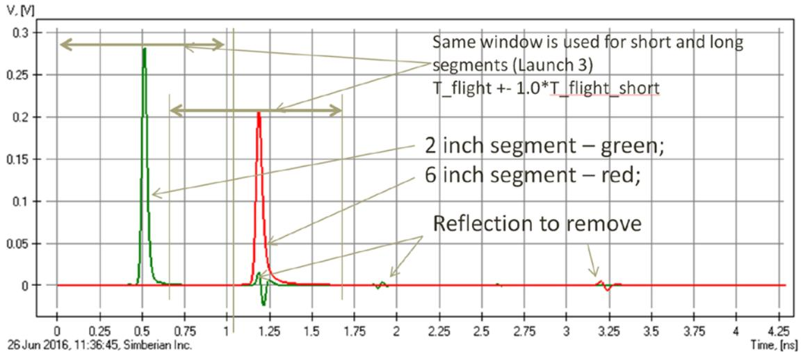
Fig. 7.6. Pulse responses of the 2 and 6 inch segments with launch 3 (bad). The oscillations caused by double reflection from the launches should be windowed as illustrated here.
