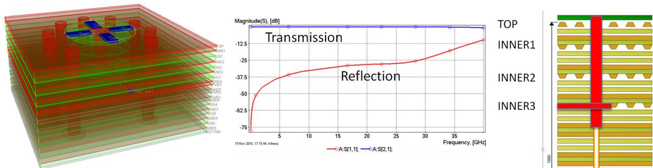
Fig. 3.6. TOP to INNER3 layer launch design for stripline structures in layer INNER2 – the reflection loss is below -20 dB up to 33 GHz and below -10 dB up to 40 GHz.
