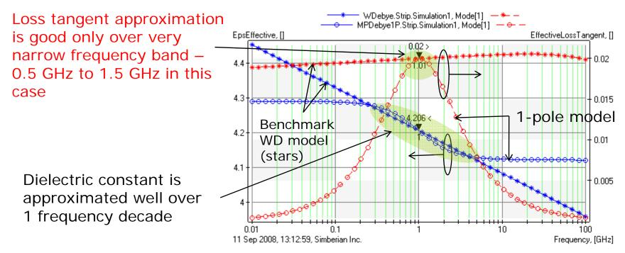
1 frequency point with DK=4.2, and LT=0.02 @ 1GHz is specified for both models
