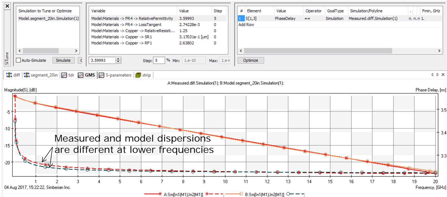
Higher measured dispersion in Phase Delay indicates that LT should be larger (dispersion)
