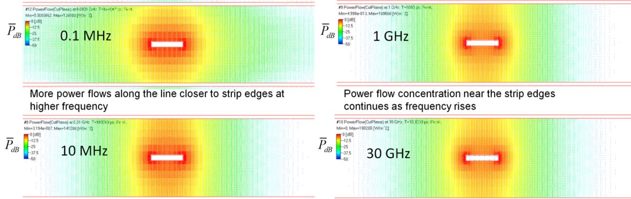
The strip is 1.2 mil thick, 7 mil wide trace, in homogeneous dielectric with  $Dk=3.76$ ,  $LT = 0.006$  @ 1 GHz, planes 0.77 mil thick and 17.2 mil apart, 1 V excitation and 50 Ohm terminators.
