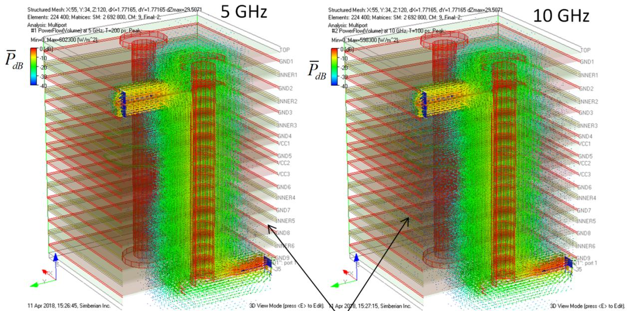
Small power leaks into inter-plane areas at lower frequencies
