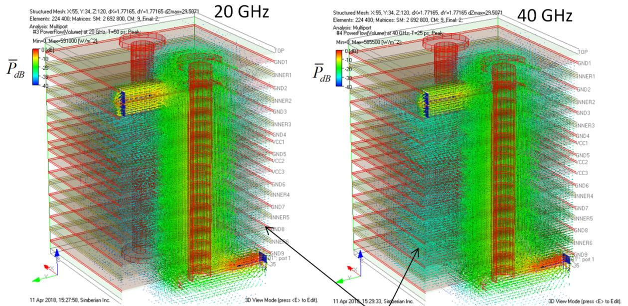
Power leaks into inter-plane areas increases with the frequency
