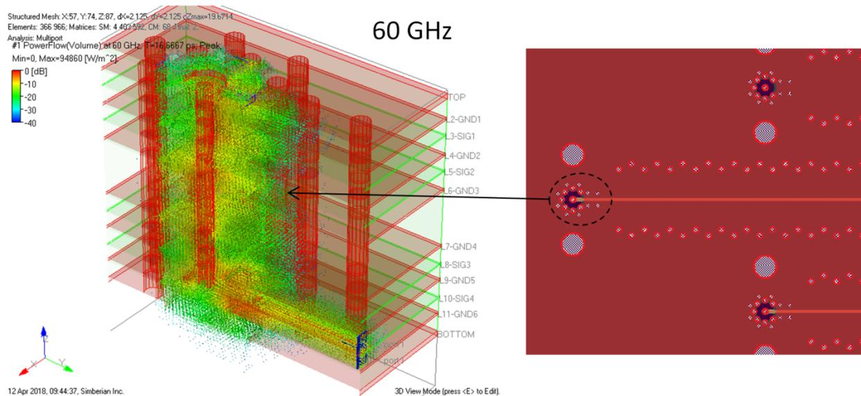
This via transition was designed by Scott McMorrow for one of our material model identification projects reported in D. Dunham, J. Lee, S. McMorrow, Y. Shlepnev, 2.4mm Design / Optimization with 50 GHz Material Characterization, DesignCon2011. It is also featured in demo-video #2018\_01 at <http://www.simberian.com/ScreenCasts.php> (demo-videos #2016\_01 and #2018\_01 use power flow density to illustrate the effect of the stitching via number and positioning).
