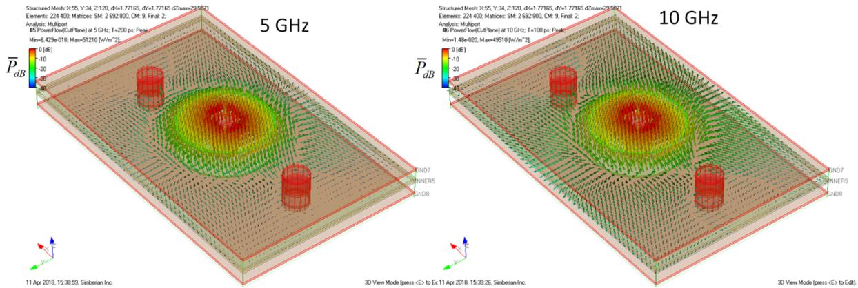
Small power leaks into inter-plane areas at lower frequencies (stitching vias work)
