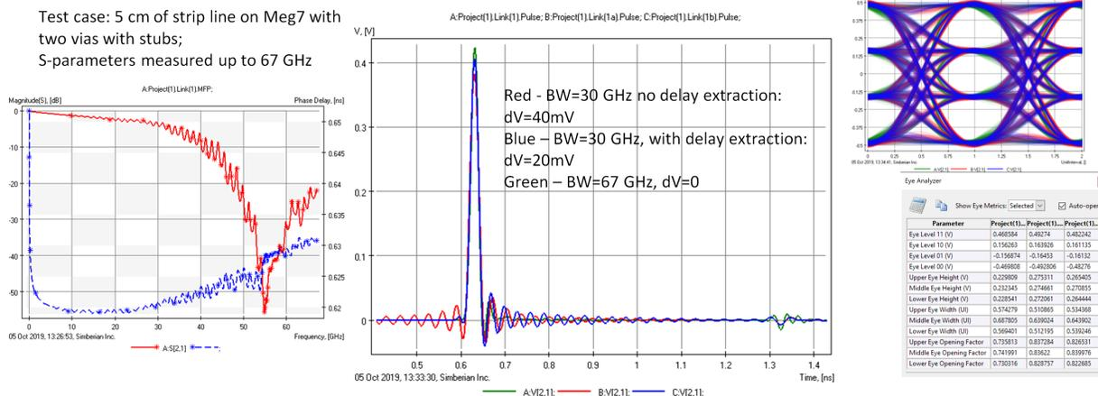
67 GHz bandwidth in this case is considered as sufficient for SSR computation and used as the benchmark – it does not produce significant error (no non-causality in the SSR). If the bandwidth is
