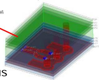
6-inch segment of t-line with inhomogeneous dielectric – non-uniform t-line model
