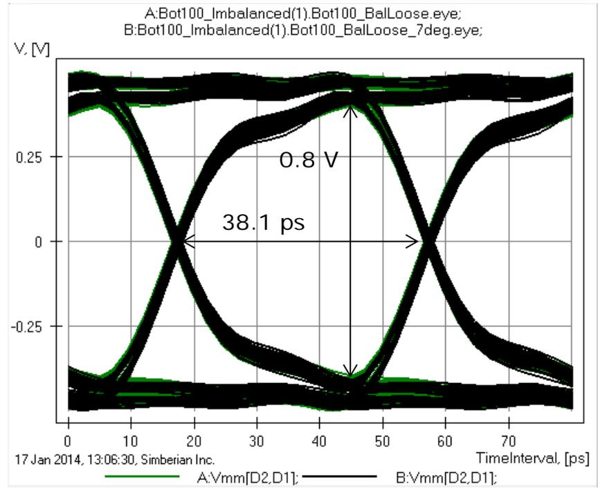
No substantial effect on jitter expected (due to narrow band of the resonance)
