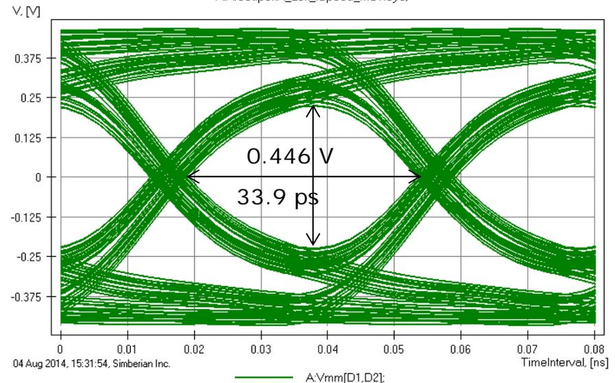
Analysis with Balanced strips produce practically the same eye (no visible difference);
