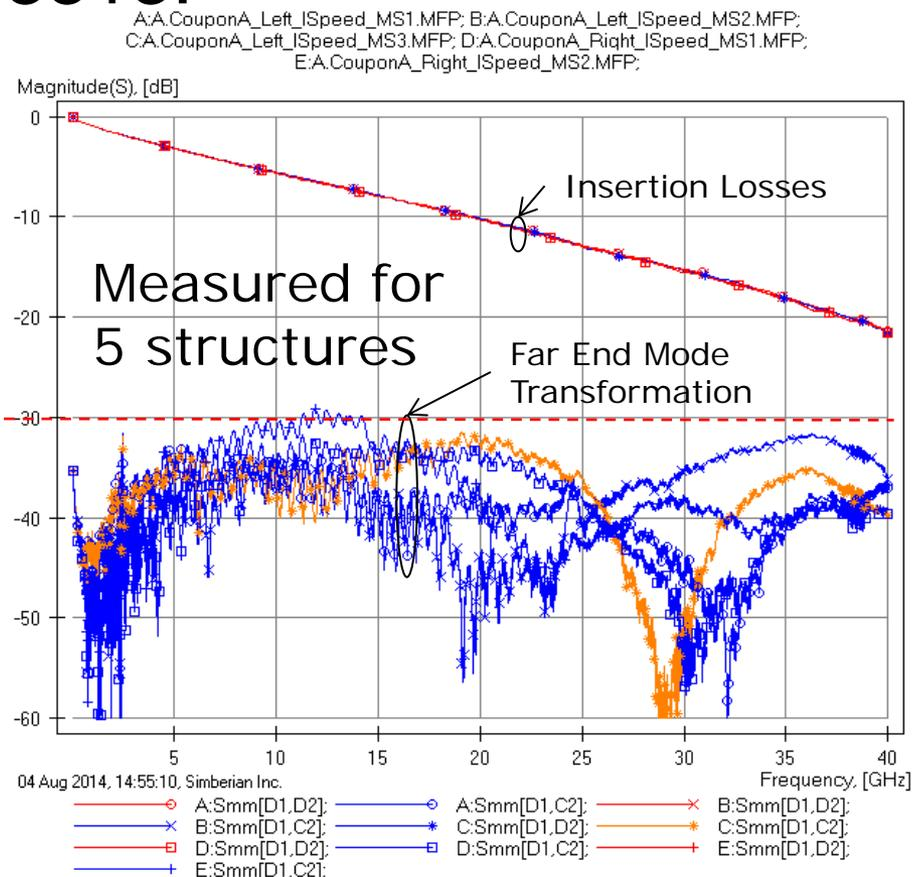
Mode transformation is smaller than expected from the TDR measurements – the imbalance is closer to 0.025
