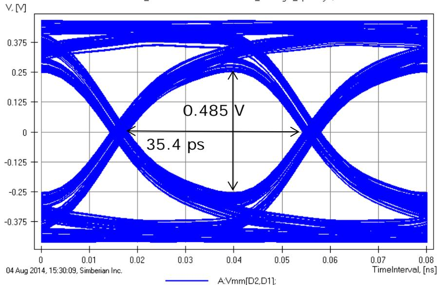
Computed from measured S-parameters for MS1 (worst case)
