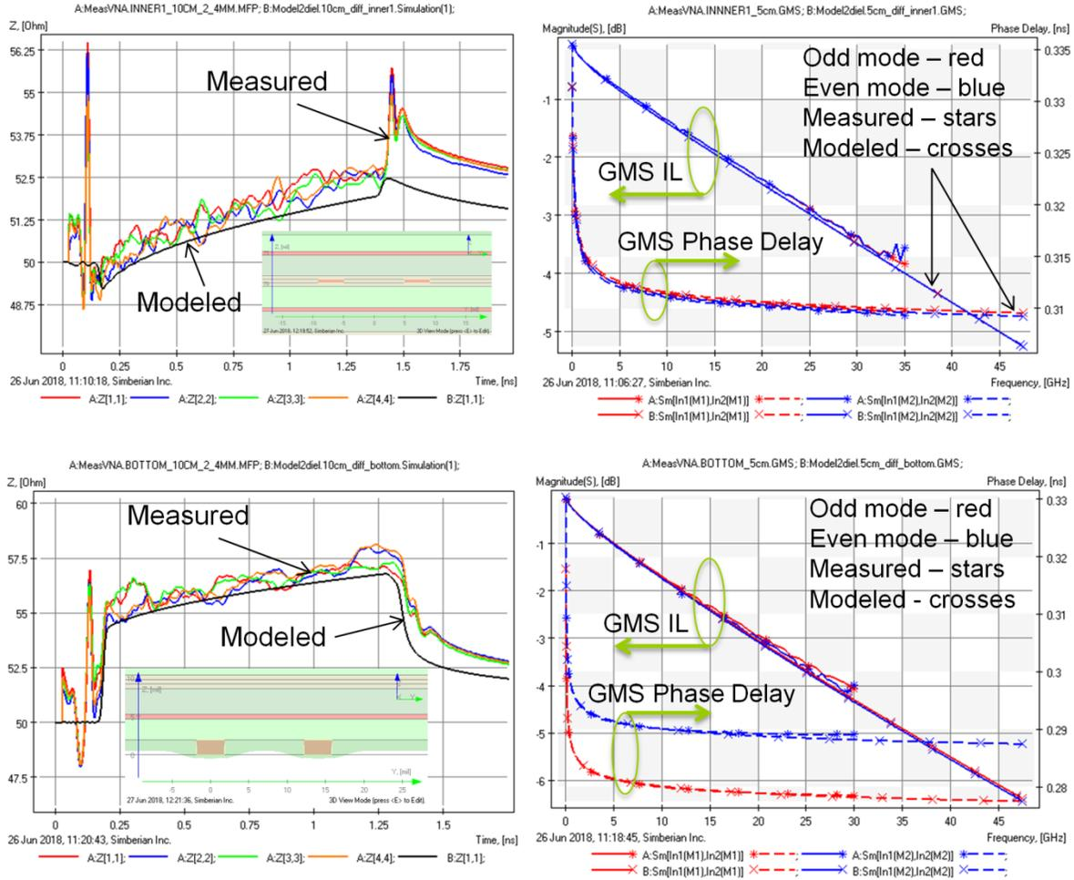
Fig. 5. TDR of 10 cm differential links measured and computed (left graphs) and GMS insertion loss (IL) and phase delay for 5 cm differential line segments measured and computed (right graphs) with the identified stackup structure and material models for layer INNER 1(top graphs) and for layer BOTTOM (bottom graphs).
