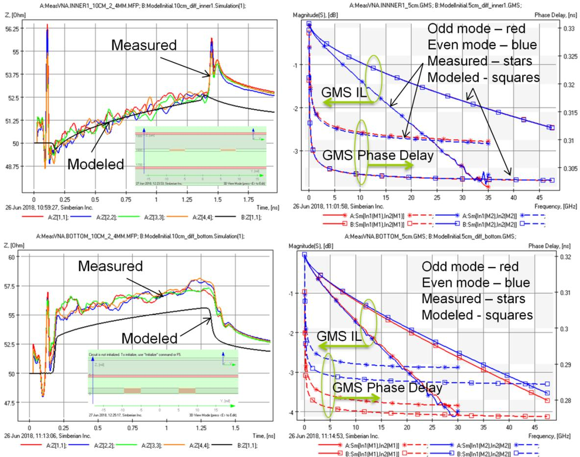
Fig. 2. TDR of 10 cm differential links measured and computed (left graphs) and GMS insertion loss (IL) and phase delay for 5 cm differential line segments measured and computed (right graphs) with the stackup structure and material parameters from the PCB manufacturer for layer INNER 1 (top graphs) and for layer BOTTOM (bottom graphs).
