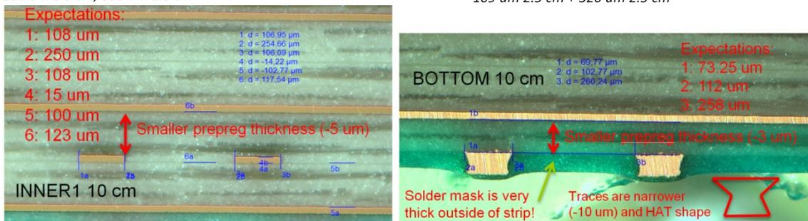
Fig. 3. Final trace geometry adjustments and example of the cross-sections of differential test links in INNER1 and BOTTOM layers (expectations are data from PCB manufacturer).
