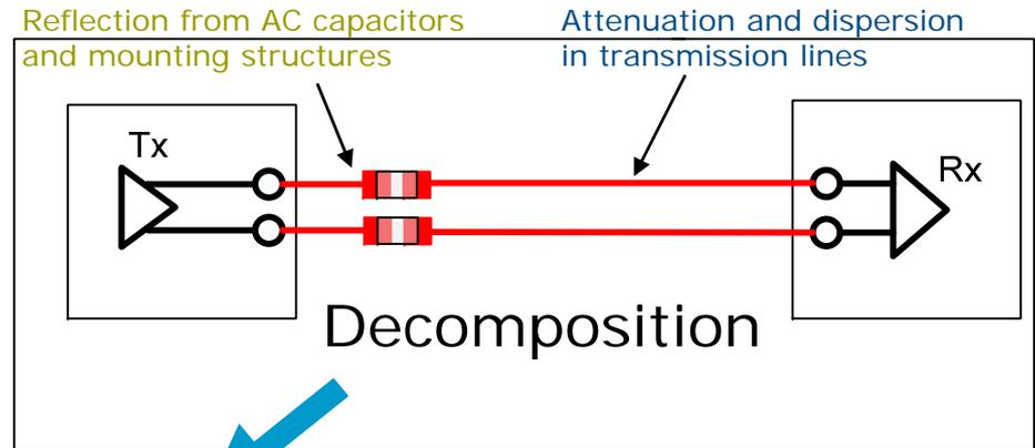
Multiport S-parameter model for the capacitors mounting structures
