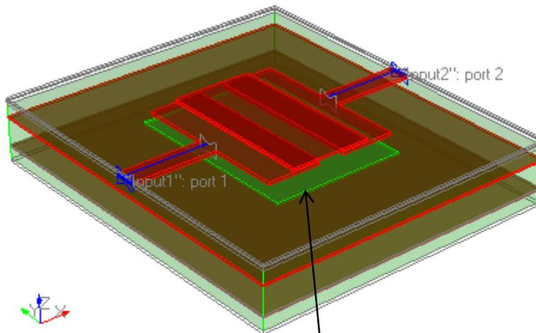
50x68 mil void in the reference plane below the capacitor mounting structure
