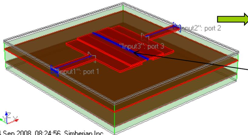
3-port broad-band S-parameter models of the mounting structures are extracted for both configurations
