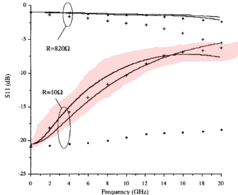
Fig. 7. Return loss versus frequency for different modelings. —: this analysis. ○○○: exact description [7]. +: measurements [7]. ■ [7].
