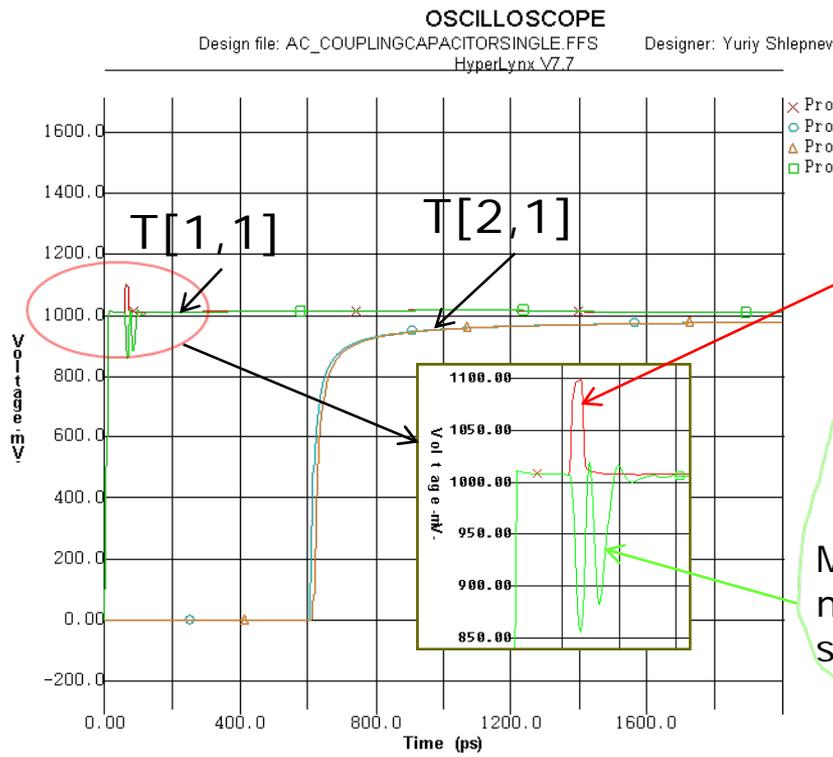
Model without the mounting structure with the capacitor model connected directly in the channel
