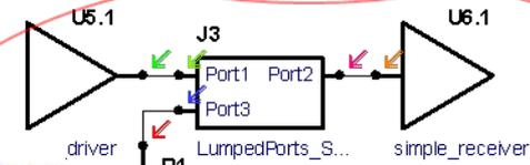
Structure with series port short-circuited by 0.1 mOhm resistor
