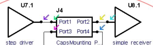
Structure with two parallel ports connected to 20-mil line segment to fill the gap
