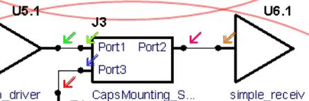
Structure with the series port short-circuited by 0.1 mOhm resistor
