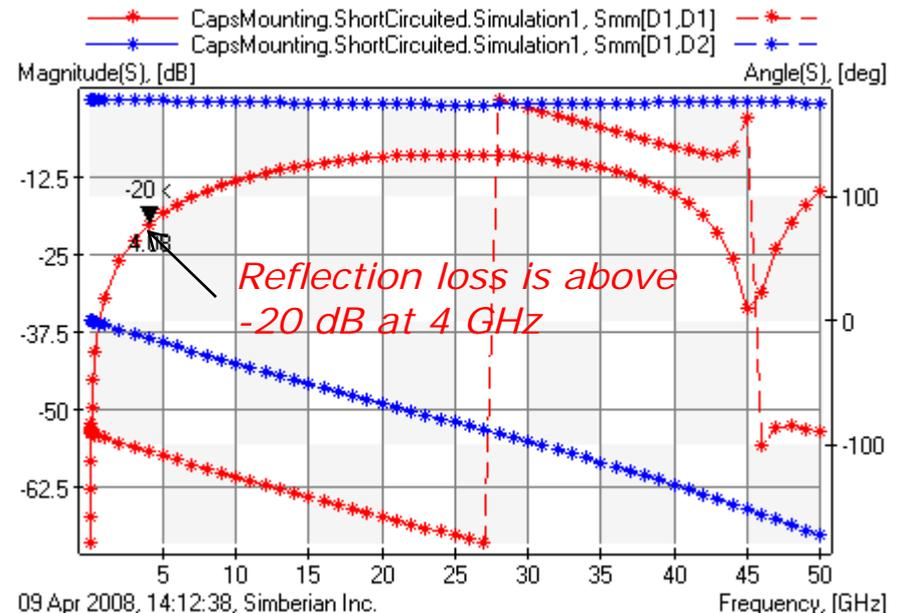
*Multipoint parameters profile has to be adjusted to see the mixed-mode S-parameters on the graph (Simulation > Results > Multipoint Parameters > Set New Profile > Input Space > Mixed Mode)*
