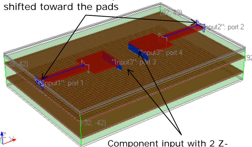
Component input with 2 Z-directed ports (Z-Ports: port 3 and 4) at the edges of the pads
