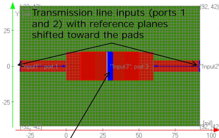
3-port broad-band S-parameter model of the mounting structure exported from Simbeor in Touchstone format
