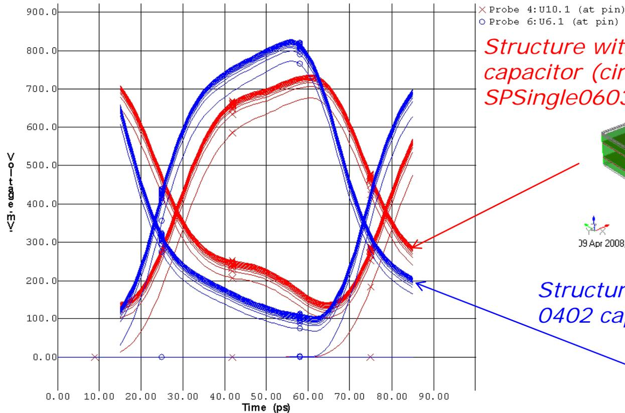
*Structure with 0603 capacitor (circuit SPSingle0603)*
