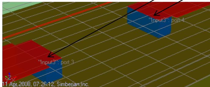
4-port model is created with transmission line ports 1 and 2 and internal ports 3 and 4
