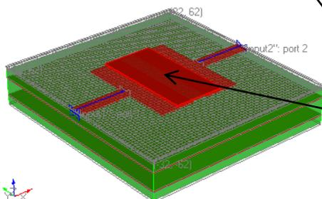
30x60 mil short-circuiting plate is slightly elevated above the board surface (layer "CapPlane")
