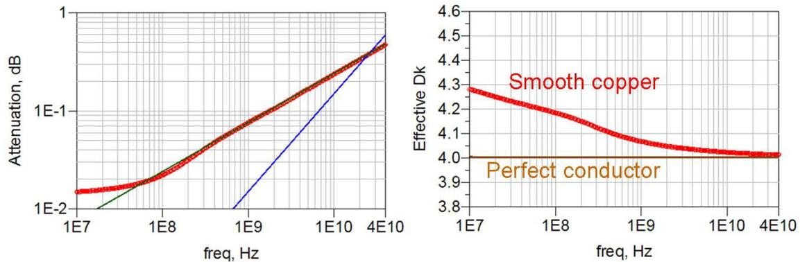
**Figure 6. Insertion loss and dispersion for smooth copper. The square root of frequency is an excellent fit to the insertion loss, while the linear dependency with frequency is a poor fit even at the highest frequency.**
