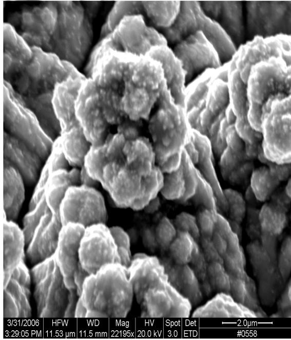
**Figure 4. SEM photograph of a High Profile surface copper Matte foil following additional “anchor nodule” electrodeposition (snowballs) on top of a heat treated base foil (with large micrograins arranged in an approximately hexagonal geographic pattern).**
