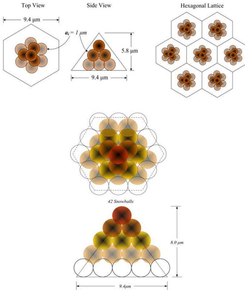
**Figure 3. Illustration of the features of the Huray model for a hexagonal Matte surface of copper upon which copper spheres have been electrodeposited. For the illustration, the spheres have been taken to be of uniform radius, but in general there is a distribution of spherical (snowball) sizes.**
