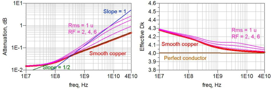
**Figure 8. Simulated insertion and effective dielectric constant for the case of lossless dielectric but surface roughness losses given by a modified Hammerstad mathematical expression in which only the scaling factor is increasing for a fixed 1 u rms peak height.**
