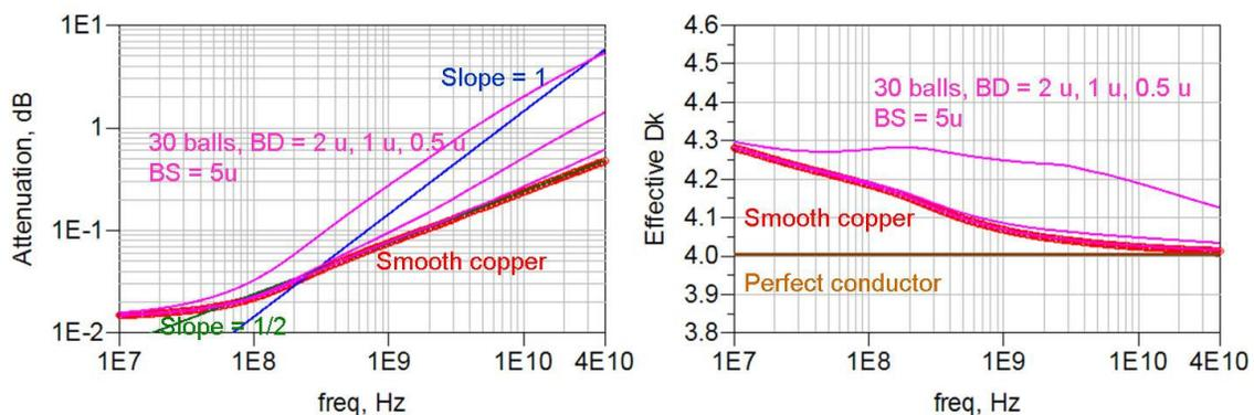
**Figure 10. Simulated insertion loss and dispersion with the Huray snowball model, changing just the ball diameter from 2 microns to 1 micron to 0.5 micron but assuming a constant base area of  $(0.5 \text{ microns})^2$  and uniform size balls.**
