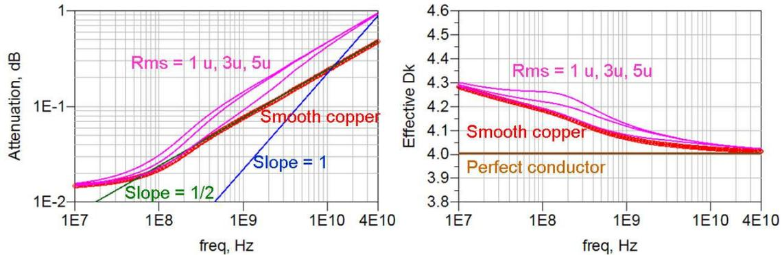
**Figure 7. Simulated insertion and effective dielectric constant for the case of lossless dielectric but surface roughness loss described by the Hammerstad mathematical equation.**
