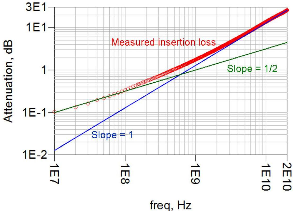
Figure 5. Measured insertion loss on a log-log scale with reference lines of slope 1 and 1/2.
