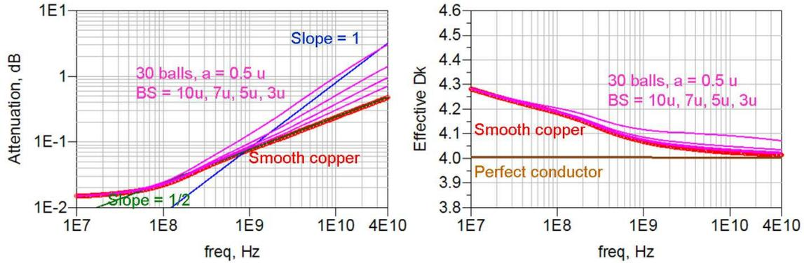
**Figure 9. Simulated results using the Huray snowball model for the case of 30 balls, each 1 micron in diameter, with different flat base areas.** I would like to see the code that deduced this chart to verify its validity.
