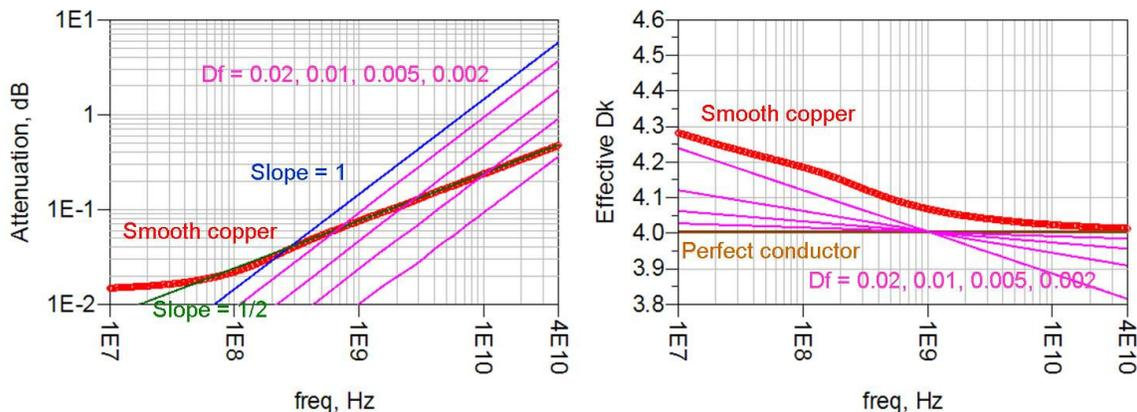
Figure 12. Simulated loss and dispersions for perfect conductor and wide band Debye model where only the Df is varied from 0.02, 0.01, 0.005, 0.002.
