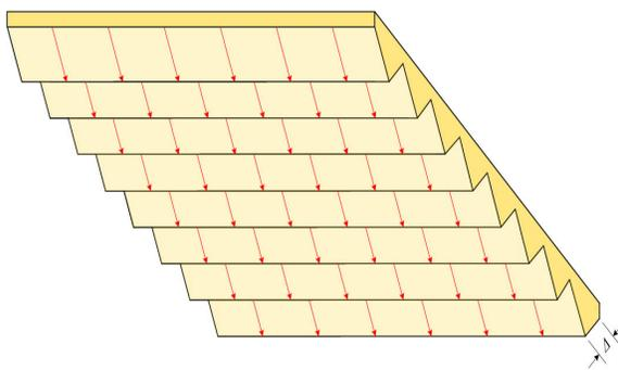
**Figure 1. Morgan's concept of transverse equilateral triangular conductor grooves on a flat base copper surface;  $\Delta$  is the RMS deviation from flatness. The red arrows show the direction of surface current flow if the signal electromagnetic field propagates from the upper left (Port 1 input) toward the lower right (Port 2 output).**
