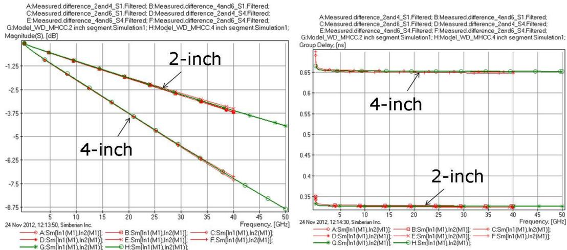
**Figure 17. Measured insertion loss and group delay for Megtron6 samples compared with the simulated values using a wideband Debye model and a modified Hammerstad approximation with values of  $Dk = 3.7$ ,  $Df = 0.002$  and  $SR = 0.3 \mu$  and  $RF = 5$ .**
