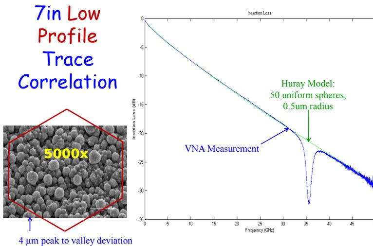
Figure 16. Insertion loss measurements on a 7 inch Low Profile trace as a function of frequency (shown in blue) compared to the Huray snowball model (in green) with the further approximations  $A_{Matte}/A_{Flat}\approx 1$  and  $N_f/A_{Flat}=50$  uniform spheres per  $(100\text{ micron})^2$  area shown in the red hexagonal structure at lower left.
