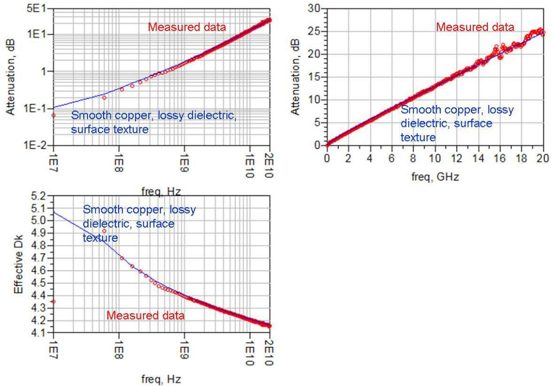
Figure 15. Final match of the measured response and simulated response using wideband Debye model, smooth copper and Huray snowball model.
