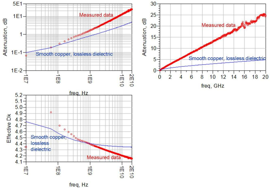
**Figure 13. Example of the measured insertion and dielectric constant for an FR4 type sample compared to the simulation using smooth copper and lossless dielectric. Note, for typical samples measured in a high volume manufacturing environment, there will be noise, especially at the low frequency and high frequency ranges.**
