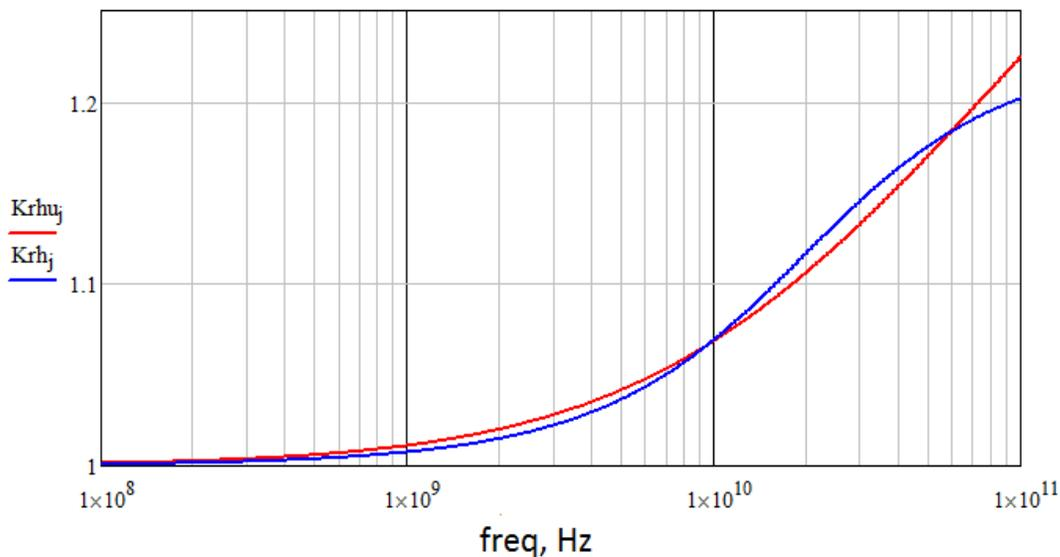
Figure 11. Huray snowball model (red line) and modified Hammerstad expression (blue line) with roughness correction coefficient matched up to 60 GHz.
