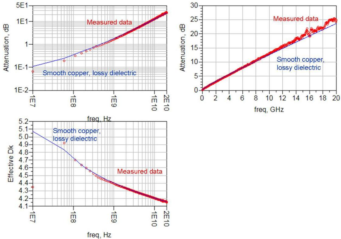
**Figure 14. Measured insertion loss and dielectric constant with smooth copper and lossy dielectric. The slight deviation at the lowest frequency is due to the difficulty of accurately measuring total attenuation less than 0.1 dB related to calibration and reproducible, low contact resistance connections.**
