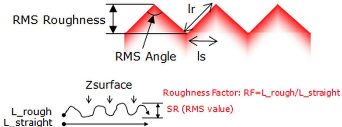
Figure 2. Illustration of the roughness factor scaling term to account for any angle of tooth and the resulting increased surface area.
