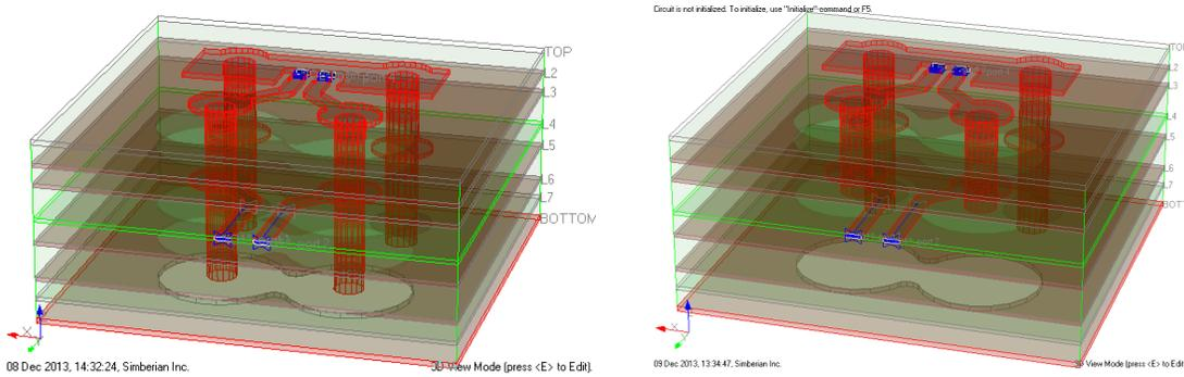
**Figure 14: 3D model of the probe launch with and without via stub. Distance between signal vias is about  $40\text{ mil}$ , distance from signal vias to stitching vias is also about  $40\text{ mil}$ . That localizes the structure only up to about  $20\text{ GHz}$ .**
