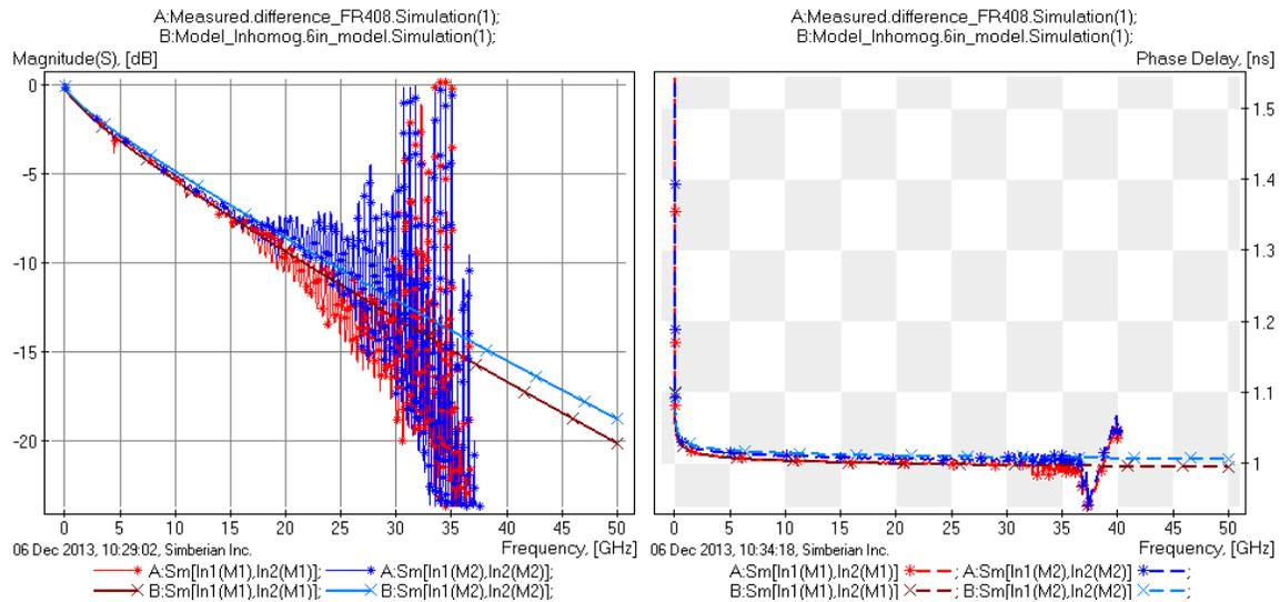
**Figure 13: Measured (lines with \*) and modelled (lines with o, cross-section from Figure 2(a), inhomogeneous dielectric model) generalized modal S-parameter: insertion loss (left graph) and phase delay (right graph) for odd mode (red and brown lines) and for even mode (blue lines).**
