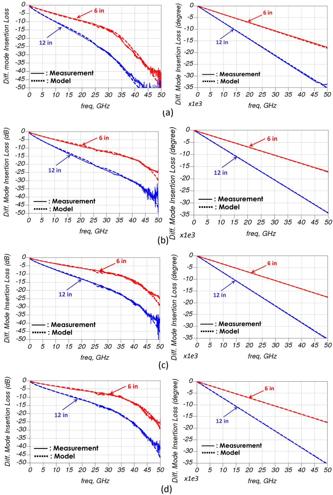
Figure 20: Magnitude and phase (unwrap) of the measured and simulated differential insertion loss for the four boards: (a) FR408HR, (b) Nelco N4000-13EPSI, (c) Megtron 6 with RTF finish, and (d) Megtron 6 with HVLP finish.
