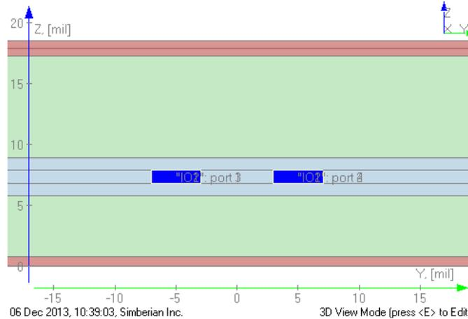
**Figure 12: Model of cross-section with inhomogeneous dielectric – blue layers are filled with resin and green with composite dielectric.**
