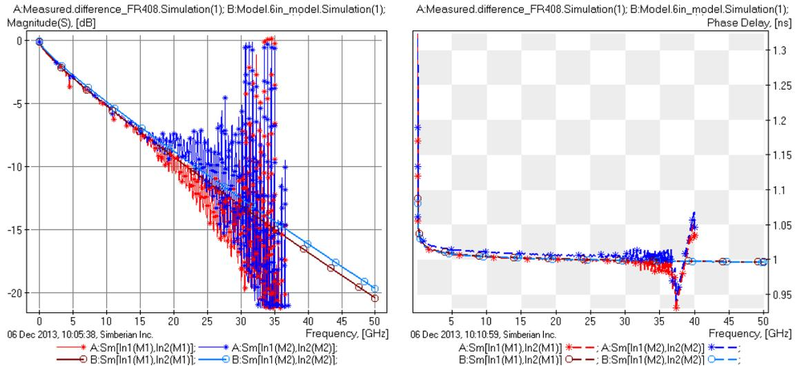
**Figure 11: Measured (lines with \*) and modeled (lines with o, cross-section from Figure 2(a), homogeneous dielectric model) generalized modal S-parameter for FR408: insertion loss (left graph) and phase delay (right graph) for odd mode (red and brown lines) and for even mode (blue lines).**
