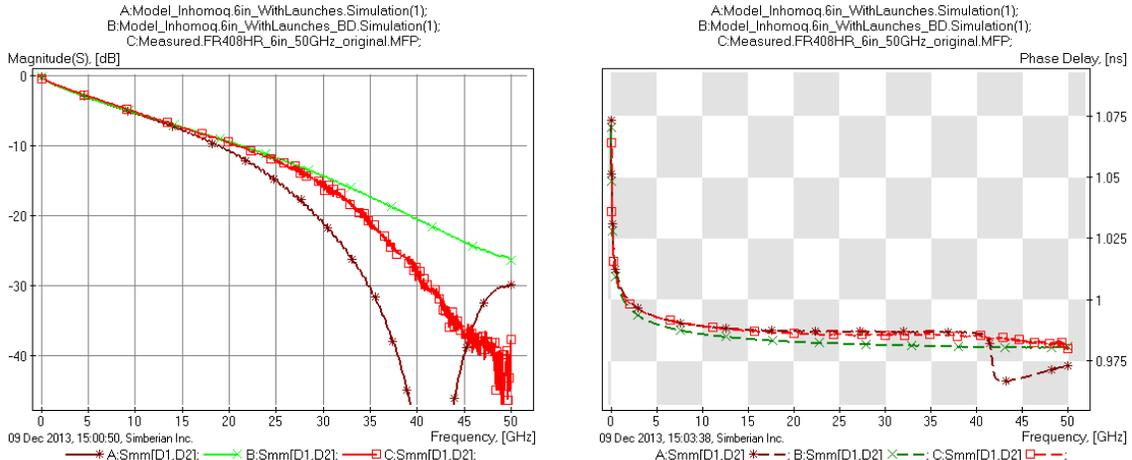
**Figure 15: Measured (red lines) and modeled with long launch via stubs (brown lines) and short via stubs (green lines) differential mode insertion losses (left graph) and phase delay (right graph) of  $6\text{ in.}$  probe-to-probe link path.**
