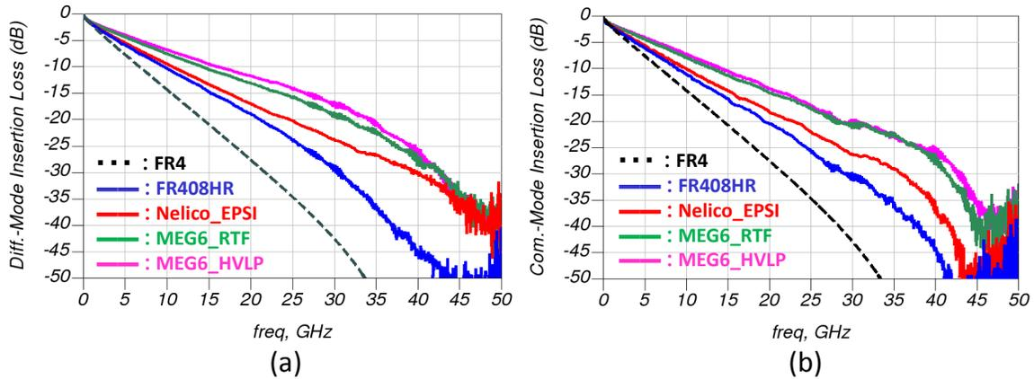
**Figure 4:** Magnitude of the measured (a) differential and (b) common-mode insertion losses are shown for the four boards: Megtron 6 HVLP (pink), Megtron 6 RTF (Green), Nelco N4000-13 EPSI (red), and FR408HR (blue). The insertion loss of typical FR-4 board is also shown from simulation (black dashed line).
