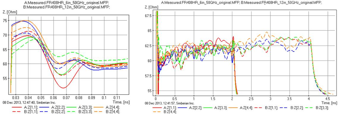
**Figure 9: TDR computed with the measured S-parameters for 6-in. (solid lines) and 12-in. (dashed lines) differential segments (20 ps Gaussian step excitation from all 4 ports). Large variations of the impedance can be observed at the launches and along the traces.**
