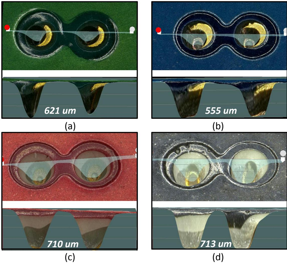
Figure 18: Top view and 3D images from a digital microscope of the back-drilled vias (holes) for (a) FR-408HR, (b) Nelco-N4000 13EPSI, (c) Megtron 6 RTF, and (d) Megtron 6 HVLP.
