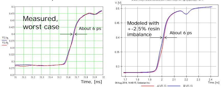
TDR measurements and simulation are done with all ports open;
