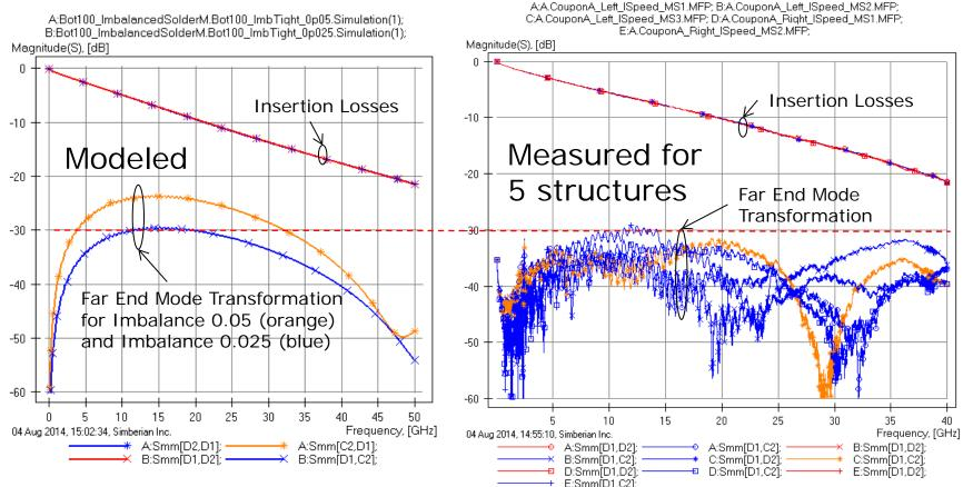
Mode transformation is smaller than expected from the TDR measurements – the imbalance is closer to 0.025
