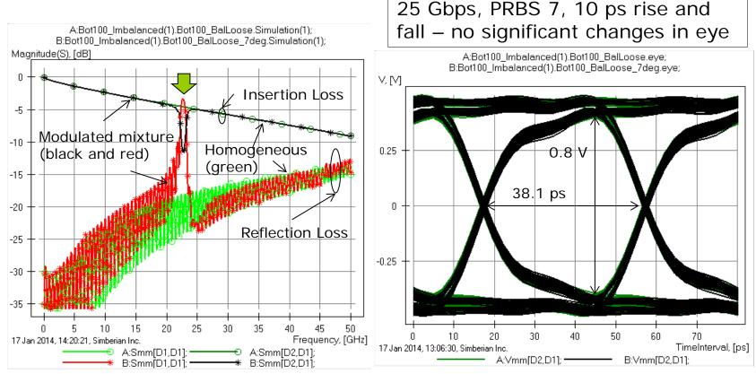
No substantial effect on jitter expected (due to narrow band of the resonance)
