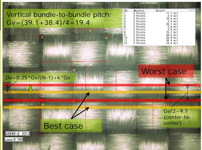
Gv=(39.1+38.4)/4=19.4 Center-to-center: Ds=9.7 Dv=0.25\*Gv/(N-1)+k\*Gv (offset) 5 samples with offset Dv=1.2+k\*19.4 mil
