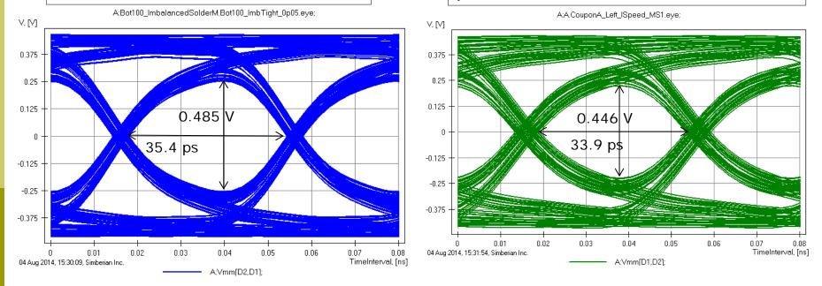
Analysis with Balanced strips produce practically the same eye (no visible difference); Why simulated and measured eyes are slightly different? – see next slide...
