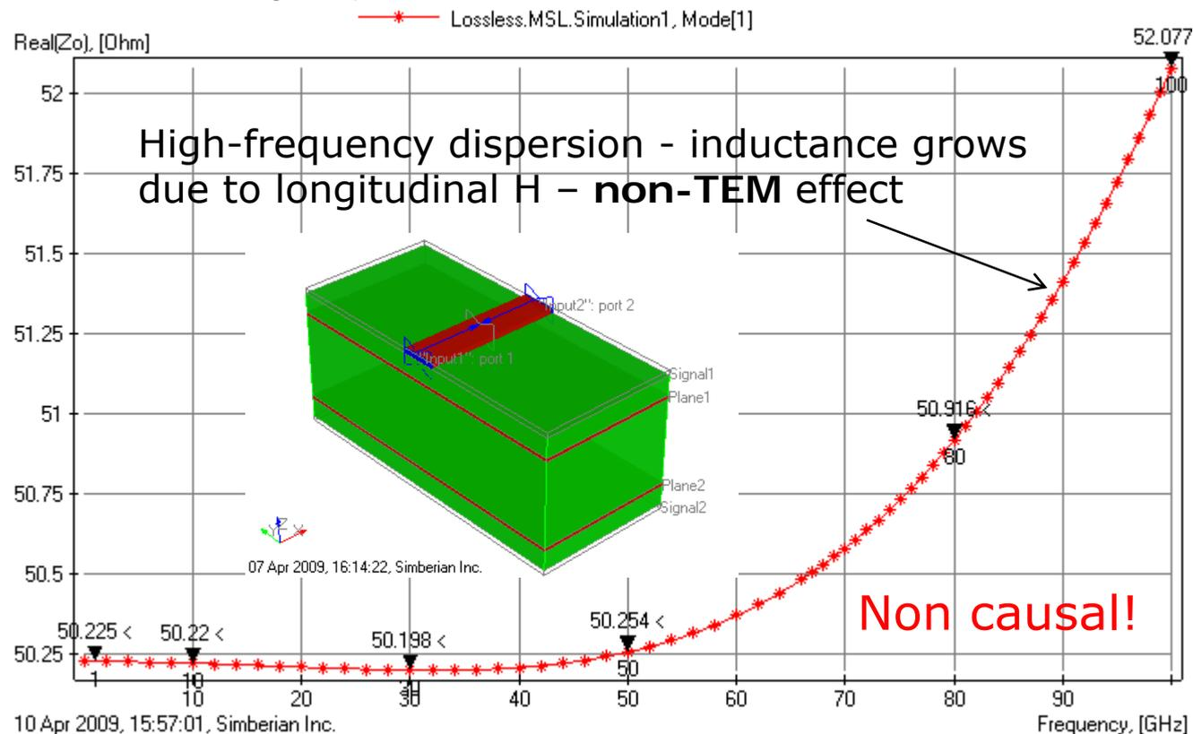
Without the high-frequency dispersion the impedance is constant or independent of frequency
