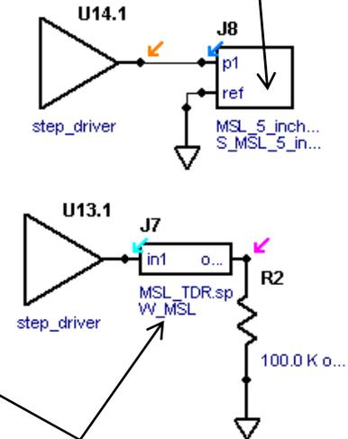
Broad-band W-element RLGC(f) model from Simbeor as SPICE sub-circuit
