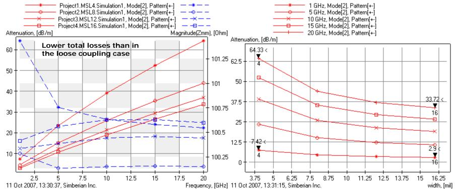
Line MSL16 with 16-mil traces has about 2.55 times smaller losses at 1 GHz and only 1.9 times smaller losses at 20 GHz than the line MSL4 with 4-mil traces. Similar to single-ended microstrip and to loosely coupled cases.
