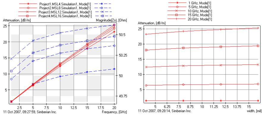
Microstrip with 16-mil trace on 8.5 mil substrate has slightly larger losses than the line with 4-mil trace on 2.3 mil substrate
