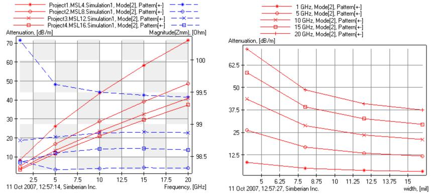
Line MSL16 with 16-mil traces has about 2.55 times smaller losses at 1 GHz and only 1.9 times smaller losses at 20 GHz than the line MSL4 with 4-mil traces. Similar to single-ended microstrip.
