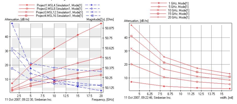
Microstrip with 16-mil trace on 8.5 mil substrate has about 3.7 times smaller losses at all frequencies than the line with 4-mil trace on 2.3 mil substrate
