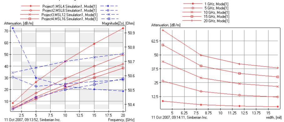
Microstrip with 16-mil trace on 8.5 mil substrate has about 2.54 times smaller losses at 1 GHz and 1.9 times smaller losses at 20 GHz than the line with 4-mil trace on 2.3 mil substrate
