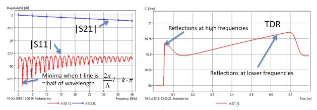
Both ends of the transmission line segment are terminated by 50 Ohm (exactly). Magnitudes of the reflection |S11| and transmission |S21| parameters are shown on the left plot and corresponding TDR on the right plot (reflection from 20 ps step response in Ohm). S-parameters are shown in dB
