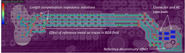
Here Simbeor evaluated effect of the cut-outs and reference pads on the impedance – those cannot be avoided. We can see that the impedance of connector and AC coupling pads is below the target and the impedance of the length compensation sections is above the target (layout mistake). The discontinuities in the reference conductors also create impedance violations (another layout mistake). Though, most of those violations may not kill the signal and are important at relatively high data rates.
