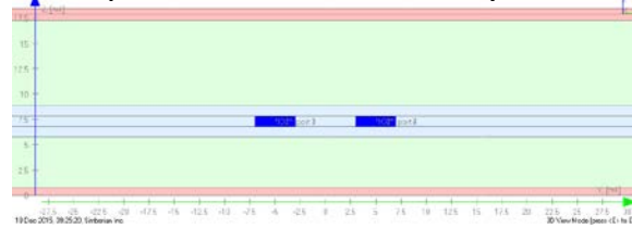
Polarization current between 2 diff. vias at 10 GHz
