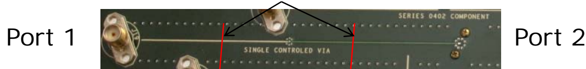
TRL Reference Planes (250 mil from stubs)
