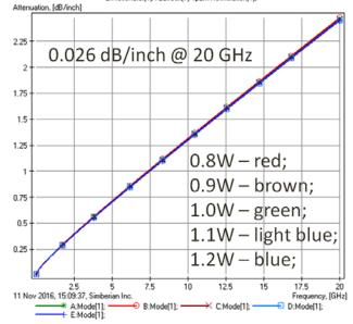
Fig. 6.3. Sensitivity of the attenuation to strip line width. 20% variation in strip width causes only 0.026 dB/inch variation in the attenuation. The dielectric loss dominates in this example.
