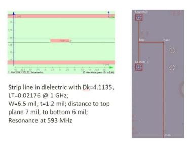
Fig. 6.1. The original geometry of T-resonator.
