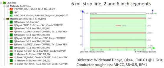
Fig. 7.1. Stackup structure and material parameters for the analysis of sensitivity of Gamma extraction to the launch design.
