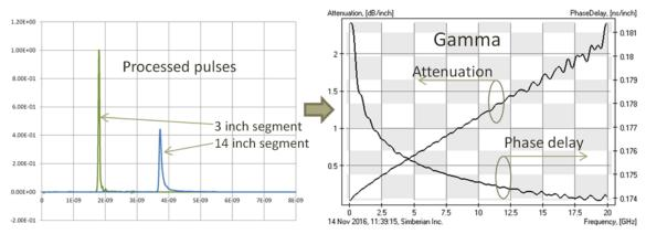
Fig. 5.4. Example of complex propagation constant extraction from two pre-processed pulse responses of 3 and 14 inch transmission line segments. Gamma is converted into attenuation in dB and phase delay to see the details.
