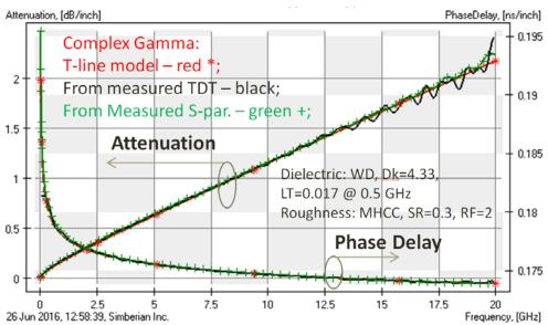
Fig. 5.8. Example of the dielectric and conductor roughness model identification with the cost-effective (from TDT) and with the precise (from S-parameters) techniques. Both techniques produced Wideband Debye model for dielectric with Dk=4.33 and LT=0.017 @ 0.5 GHz and Modified Hammerstad Correction Coefficient (MHCC) with SR=0.3 and RF=2 for the conductor roughness.
