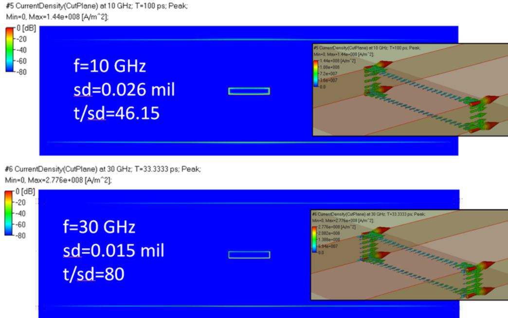
Fig. 9. Current density distribution in strip and planes of symmetric strip line at high frequencies – current flows in extremely thin layer and higher current density is observed in the conductor corners.
