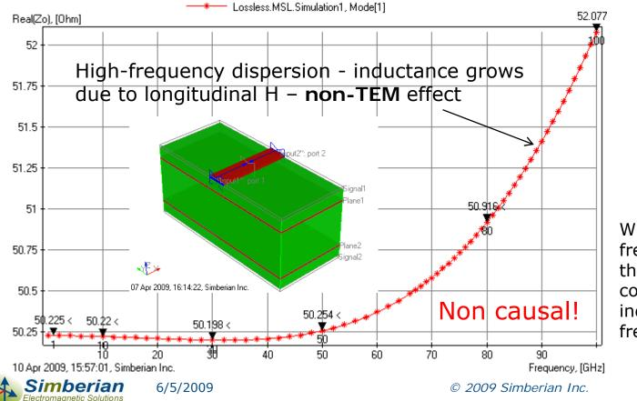
Without the highfrequency dispersion the impedance is constant or independent of frequency
