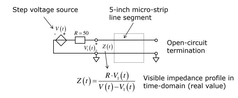
Using step source with different rise times we should be able to see the reflection from characteristic impedance of t-line before the wave is reflected from the open end (about 1.4 ns)
