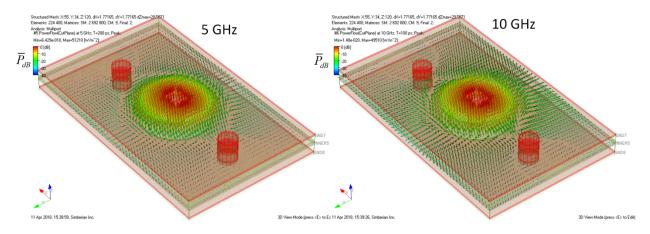
Small power leaks into inter-plane areas at lower frequencies (stitching vias work)
