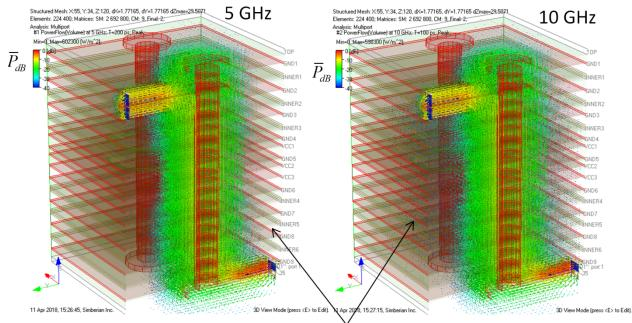
Small power leaks into inter-plane areas at lower frequencies
