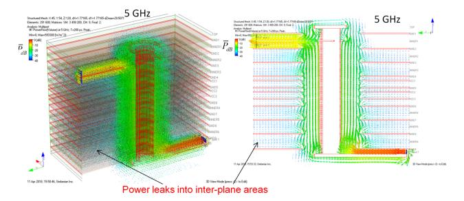
This model uses absorbing boundary conditions on the outside boundaries of the simulation domain – it absorbs the energy of the parallel plane waves going from the via. For instance, here is the close up of what is going on between the reference planes GND7 and GND8 – the power flows along the via in the anti-pad area and flows mostly outward between the parallel planes and is absorbed at the outer boundary:
