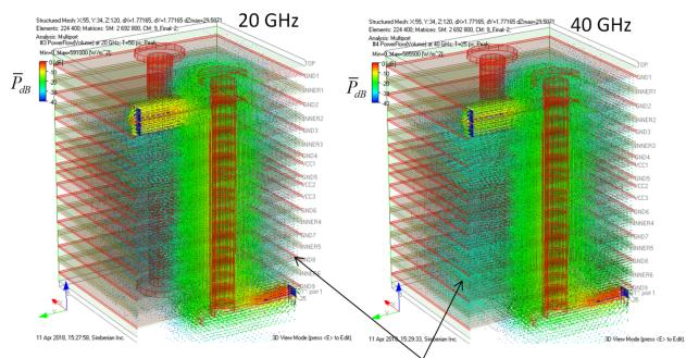
Power leaks into inter-plane areas increases with the frequency
