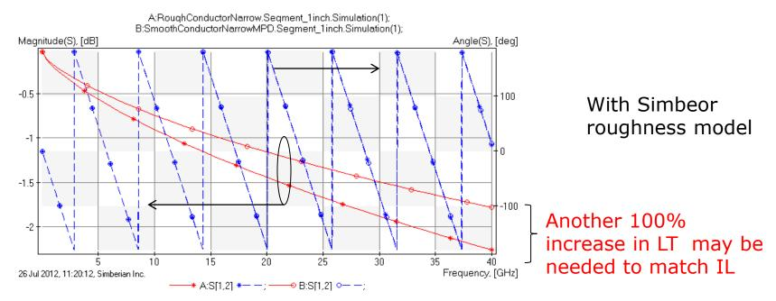
Model with rough conductor - stars Model with smooth conductor and new dielectric - circles
