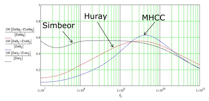
Less then 0.6% difference – not significant! We can move roughness effect into dielectric model for high-loss dielectrics
