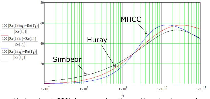
Up to about 60% increase in attenuation due to roughness
