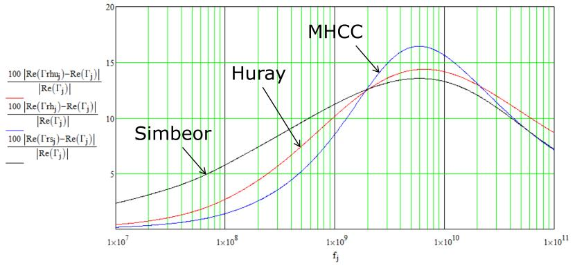
Up to about 15% increase in attenuation due to roughness
