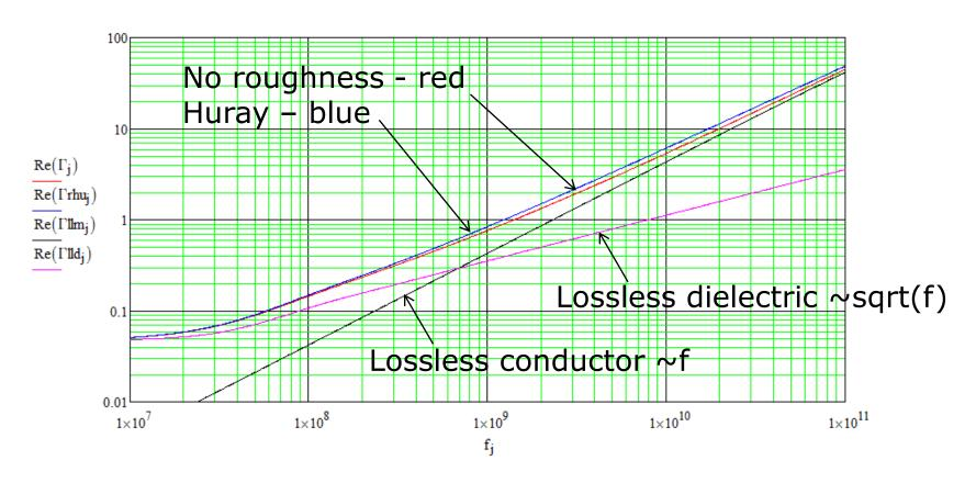
All other roughness models produce  $\Gamma$  very close to Huray model Absolute values for different roughness models is difficult to compare – relative can be used
