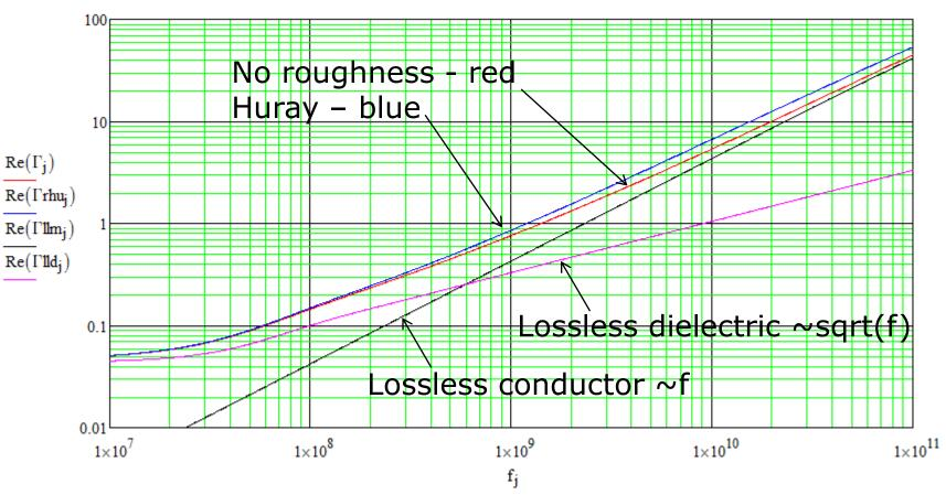
All other roughness models produce Γ close to Huray model and do not confirm linear attenuation growth concept All other conclusions are similar to the case of regular copper
