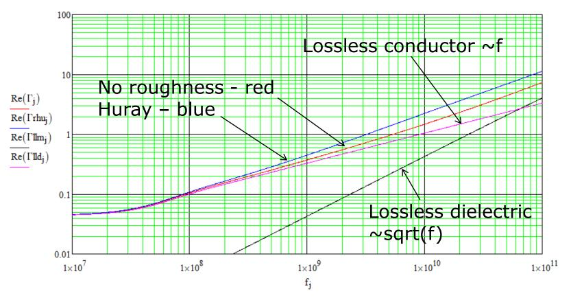
All other roughness models produce  $\Gamma$  very close to Huray model Again, let's compare relative differences between roughness models
