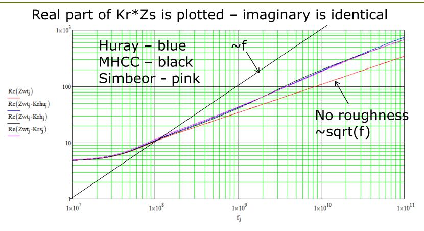
Non of the models predicts change of asymptotes from sqrt(f) to linear (typical roughness parameters)
