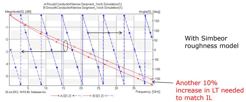
Model with rough conductor - stars Model with smooth conductor and new dielectric - circles
