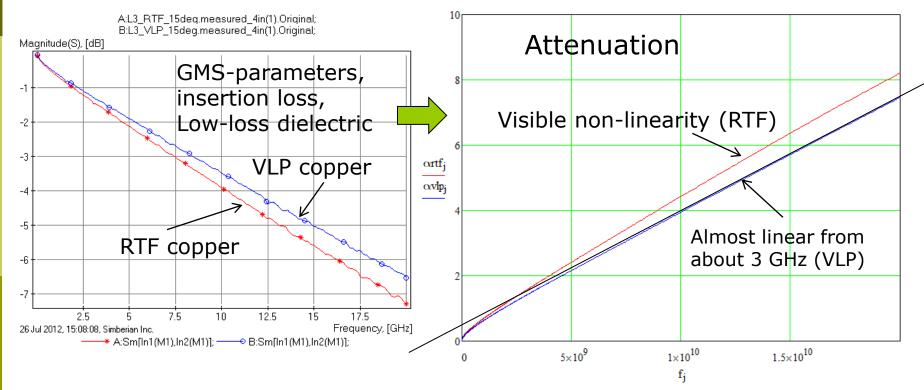
Though, there is something in this linearity above 3 GHz for copper with very low profile copper – may be not much roughness effect?
