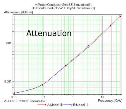
Model with rough conductor - red lines with stars Model with new dielectric – blue lines with circles
