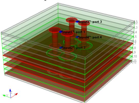
Extract only differential to differential multiport parameters, normalize Sparameters to 100 Ohm
