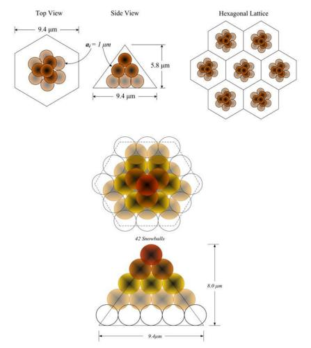
Figure 3. Illustration of the features of the Huray model for a hexagonal Matte surface of copper upon which copper spheres have been electrodeposited. For the illustration, the spheres have been taken to be of uniform radius, but in general there is a distribution of spherical (snowball) sizes.
