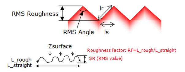
Figure 2. Illustration of the roughness factor scaling term to account for any angle of tooth and the resulting increased surface area.
