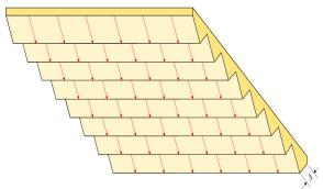
Figure 1. Morgan's concept of transverse equilateral triangular conductor grooves on a flat base copper surface;  $\Delta$  is the RMS deviation from flatness. The red arrows show the direction of surface current flow if the signal electromagnetic field propagates from the upper left (Port 1 input) toward the lower right (Port 2 output).
