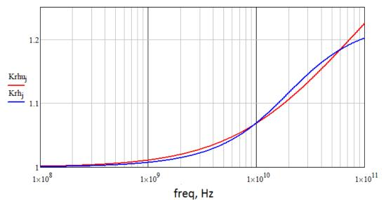
Figure 11. Huray snowball model (red line) and modified Hammerstadt expression (blue line) with roughness correction coefficient matched up to 60 GHz.
