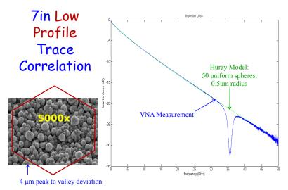
Figure 16. Insertion loss measurements on a 7 inch Low Profile trace as a function of frequency (shown in blue) compared to the Huray snowball model (in green) with the further approximations  $A_{Matte}/A_{Flat}\approx 1$  and  $N_i/A_{Flat}=50$  uniform spheres per (100 micron)<sup>2</sup> area shown in the red hexagonal structure at lower left.
